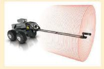
way to get that interior geometric data, and pretty much the only way." Other applications include documenting pipe wall deterioration for planned maintenance, repair and relining.
