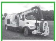
2003 Sterling L7500 Vac Truck: CAT 3125 @ 315 hp, A/T, 55k miles, spring susp., 2003 Vac-Con V390LHAD, 3 compressor fans, 10' telescopic boom, HS drive, articulating hose reel, hi-dump debris tank.....\$79,500
