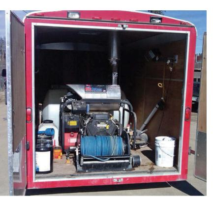
The HotJet USA hot-water jetter produces about 2,800 psi at a maximum of 25 gpm, helping workers thaw frozen sewer lines much more efficiently.
