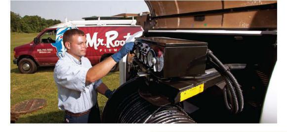
Mr. Rooter of Hudson Valley's plumbers also have access to a TRIC Tools pipe bursting system and a Perma-Liner pipelining system when they have to deal with a damaged sewer
