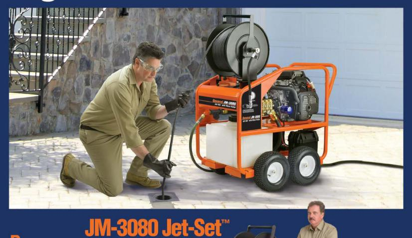
need it – even in hard to reach places. The powerful JM-3080 blasts grease, sediment and ice from 4" to 8" lines up to 300 ft. long. Tip the trim, precisely balanced jet onto the rear wheels and one person can easily maneuver it into position. Try that with a trailer jet! With a removable 300 ft. capacity hose reel, 20 hp (614 cc) Honda engine and 3000 psi/8 gpm pump, the JM-3080 is like a trailer jet – without the trailer!
