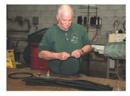
ABOVE: Rick Chapman puts together a gasket seal for a lateral pipe liner. RIGHT: Dave Laman sews a flange for a felt pipe liner.
