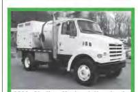
2002 Sterling Vactor jetter truck: 3126 CAT, Allison auto., Vactor V-8015 ram jet, 1,500-gallon water, 80 gpm pump, 2,500 psi, 85,947 miles, 3,932 hours, 649 P.T.O hours, ex-municipal truck.
