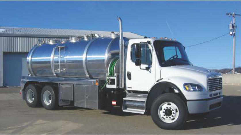
A pump truck featuring a full-sized jetting unit capable of handling jobs that require high pressure and flow.
