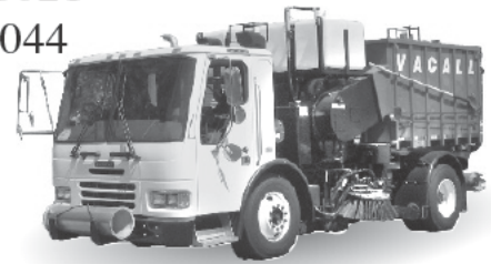
2008 Condor, dual steer truck mounted, large capacity sweeper with dual sweep gear and catch basin cleaner unit Price by Request
