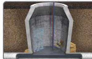
Curtain grouting with wand
