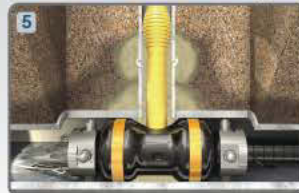
Lateral packer injecting grout
