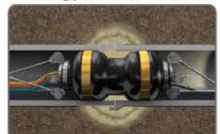
Chemical grout injected into soil
