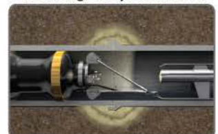
Grout collar stops infiltration
