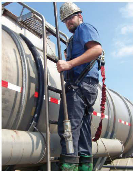
Bastrop technician Stormy Bridges climbs onto a tanker trailer with a Gamajet V high-pressure cleaning nozzle. (Photo courtesy of Bastrop Tank Wash)
