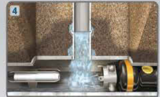
Water infiltration at lateral
