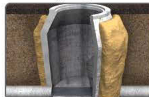
Grout curtain stops infiltration
