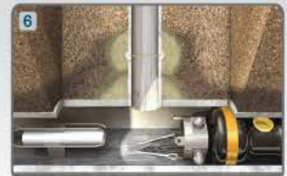
Grout collar stops infiltration
