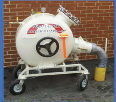
Perma-Lateral™ Air Inversion & Pull In Place
