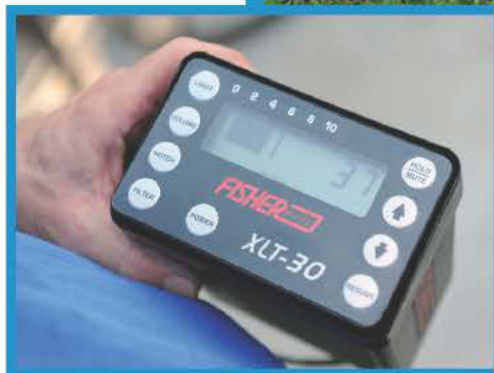
Leak detector Mark Hartstein, left, and senior leak detector Dave Richardson use a leak detector from Fisher Research Lab to locate a leak underneath a concrete slab. (Photography by Cliff McBride)
