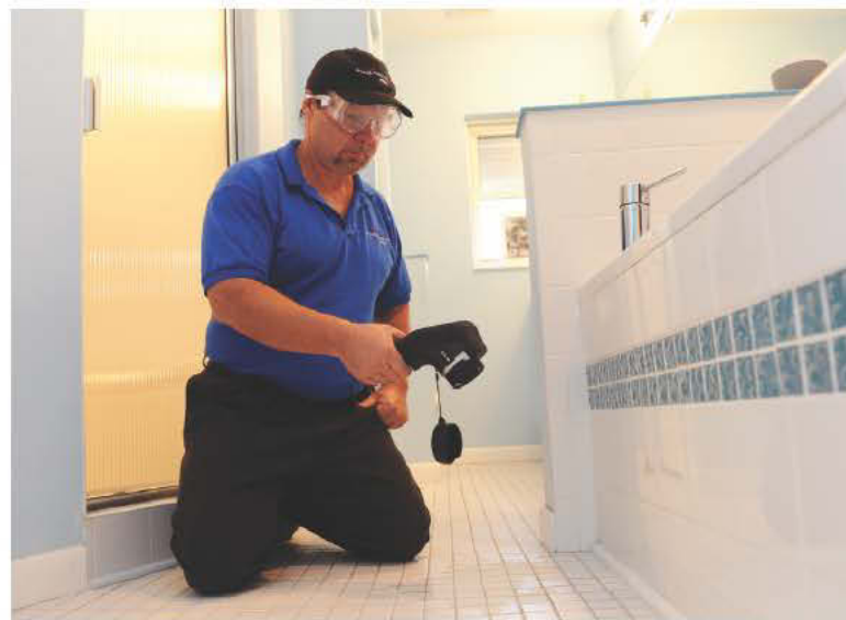
LEFT: Sewer jetting technician Chris Abbott uses a RIDGID SeeSnake to ensure a sewer pipe is clean and clear of debris after jetting. ABOVE: Senior leak locator Dave Richardson uses a FLIR E40bx infrared camera to identify areas of moisture in a bathroom.
