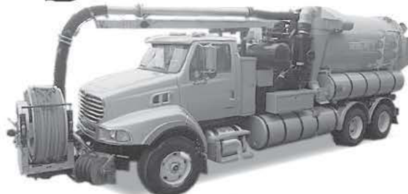
2007 Sterling/Vactor 2115, 18" PD, 80 GPM/2,500 PSI, Accumulator, Multiflow, tele rotating reel, low hours and miles.
