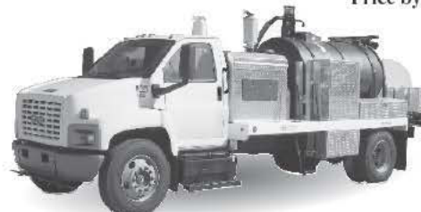
2006 GMC (very low mileage) truck mounted high pressure jetter unit with TV inspection and vacuum system Price by Request
