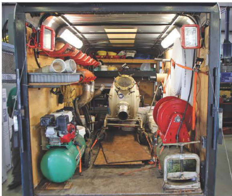
A view inside the Perma-Liner lateral replacement system trailer.
