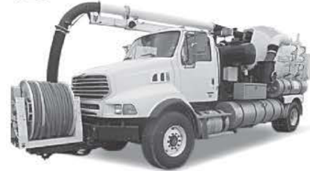
2006 Vactor 2110, 80 GPM/2,500 PSI, Multiflow, Accumulator, 1,000 Gallon water capacity, 8' teleboom, Rotating hose reel, Roots 824 blower, 2006 Sterling, 350 HP, Automatic transmission, 66,500 Miles/4,600 hours.
