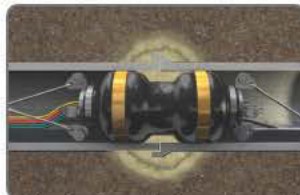
Chemical grout injected into soil
