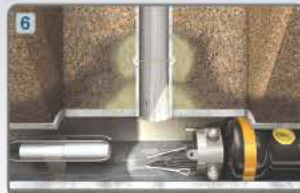
Grout collar stops infiltration
