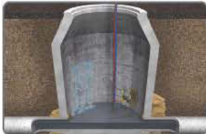
Curtain grouting with wand
