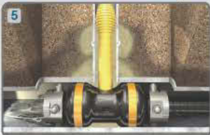
Lateral packer injecting grout
