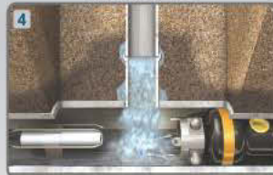
Water infiltration at lateral
