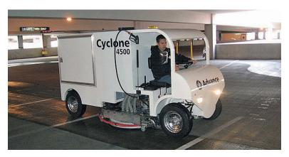
The Advance brand Cyclone surface cleaner can carry 240 gallons of water and deliver the cleaning power of 4,000 psi at a flow of 6 gpm. The unit also sucks up water and debris, eliminating dirty water runoff.
