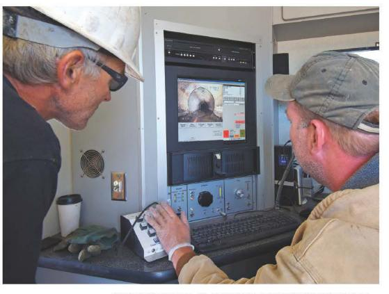
ABOVE: David Scheele, left, and Blake Hovey view the interior of a stormwater pipe on an RS Technical Services camera inspection system. BELOW: Kelly Wright helps measure where the jet rodder will be placed in a storm drain.
