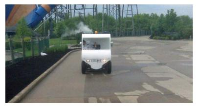
A member of the Contract Sweepers crew keeps a close eye on the pavement from the cab of the Cyclone surface cleaner.
