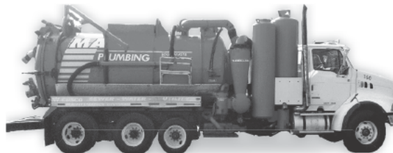
3163V 4000 U.S. gallon 2 compartment carbon steel 3700 waste, stainless steel 300 water Cusco D.O.T. Turbovac 3827 D.C. series mounted on a 1999 Sterling
