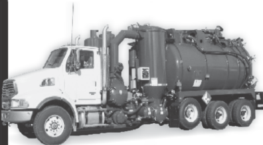
4931C POWERVAC 3800, 3,250 U.S. gallon, carbon steel vacuum tanker with a Hibon PD blower 3800 SCFM with vacuum to 27" mercury. Dump type; D.O.T. 407/412 regulations
