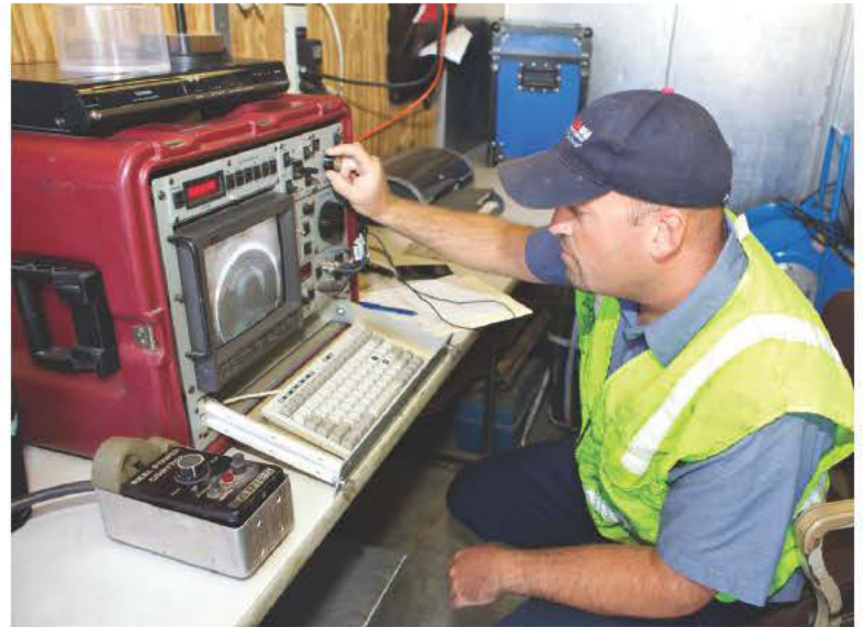
LEFT: Jason Langlais, left, and Christopher Daigle pull the Aries camera out of a manhole after inspection. RIGHT: Jason Langlais operates the Aries camera inspection equipment from inside the CCTV truck.
