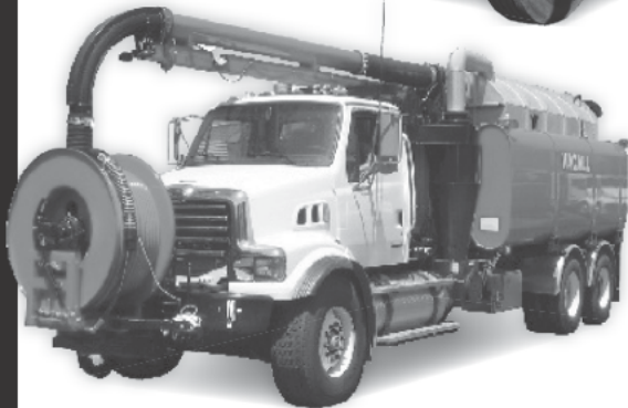
13366V 2008 Sterling LT7501 with a VacAll AJV1015; 10 yard debris body, 1500 gallon water, Combination Vacuum/Jetting unit. Pre-owned Rental Unit
