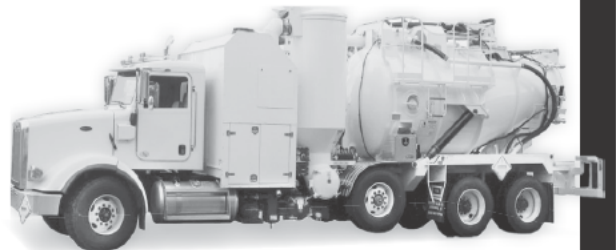
13478V POWERVAC 3800, 3,000 U.S. gallon, carbon steel vacuum tanker with a Hibon PD blower 3800 SCFM with vacuum to 28" mercury. High dump type; D.O.T. 407/412 regulations
