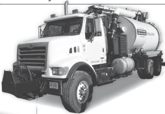
5850V 2001 Sterling cab and chassis Vactor series 2112 Hydroexcavator
