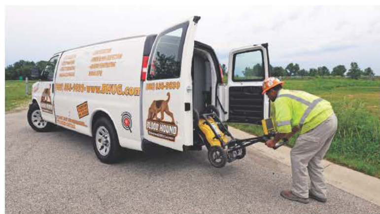
Above: Utility locating specialist Dwayne Ware catches underground data with the Trimble GeoExplorer 6000. Right: Ware gets the Sensors & Software Noggin ground penetrating radar (GPR) unit ready for a job.
