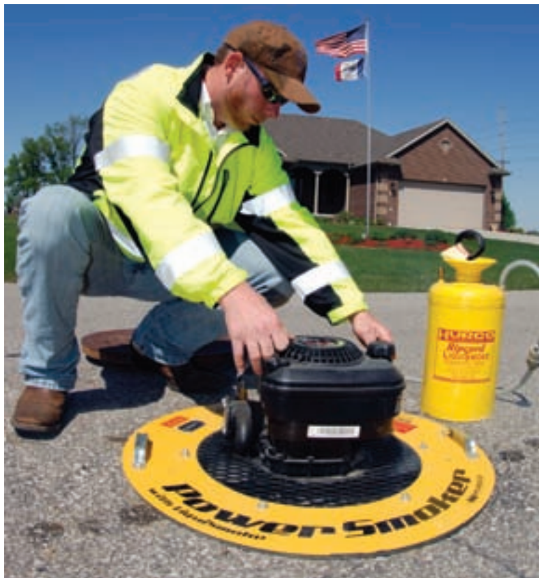
Shane Jacobson sets a Power Smoker (Hurco Technologies) for a smoke test. RIGHT PHOTO: Phil and Nick Paulson lower a camera and Badger transporter from Aries Industries.
