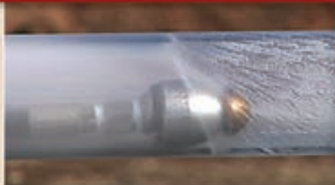
High-speed rotation improves unplugging and root removal.
