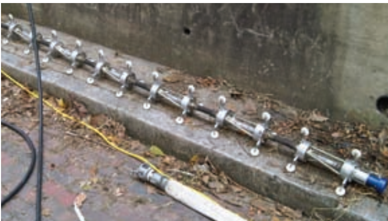
The 13-foot-long Light Train for liner curing has eight 400-watt ultraviolet bulbs.
