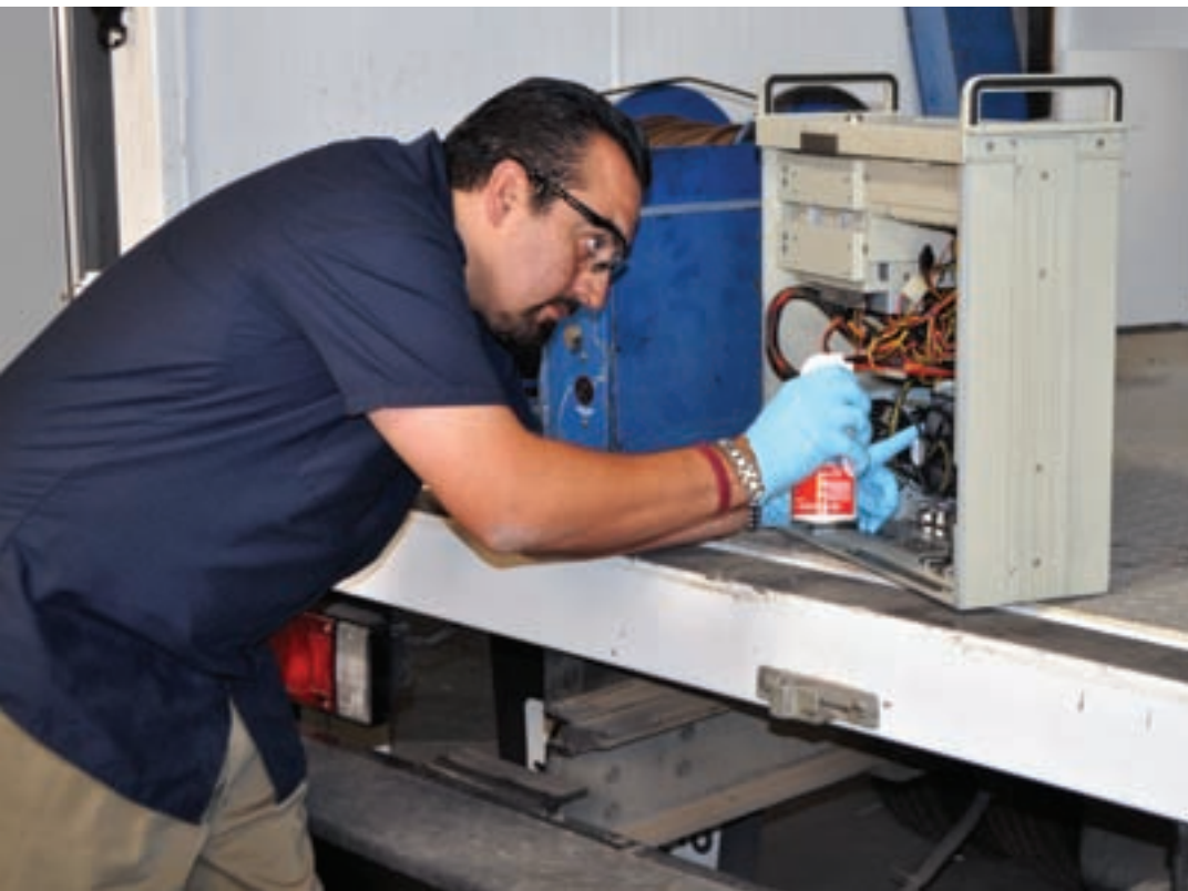
Sean Trammel, operations manager at Innerline Engineering, cleans out the interior of a CCTV inspection computer.
