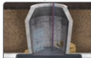
Curtain grouting with wand
