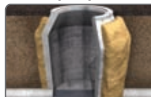
Grout curtain stops infiltration
