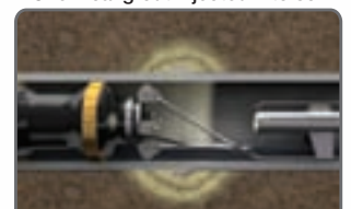
Grout collar stops infiltration
