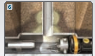
Grout collar stops infiltration
