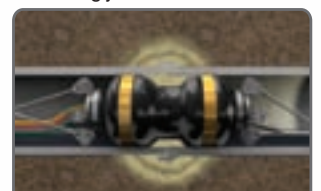
Chemical grout injected into soil
