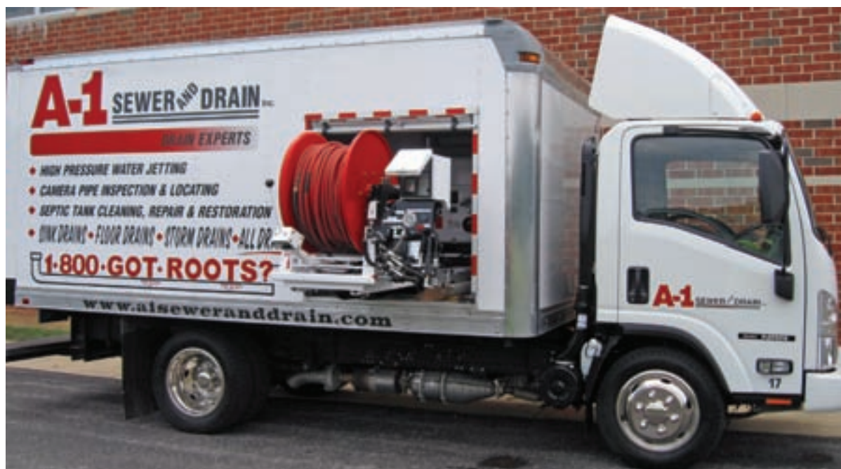
The truck has a 14-foot insulated Kold King box body from Supreme Corp., a cab-forward design, a retractable and articulating hose reel with 500 feet of 1/2-inch hose, a high-pressure jetter that generates 4,000 psi/18 gpm, and two 150-gallon water tanks. (Photo courtesy of A-1 Sewer and Drain)
