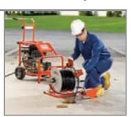
ates tight turns. The hose reel detaches from the cart for loading into service vehicles and carries 200 feet of 3/8-inch hose.
