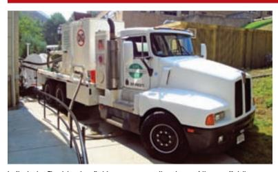
Left photo: The blue lay-flat hoses go over the drum of the scaffolding and into the liner, while the 4-inch black hoses discharge and recirculate water from the boiler. Right photo: The front of the 12-million-Btu boiler truck. (Photos courtesy of Advanced Pipe Inspection)
