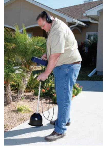
Master plumber Derek Simons uses the Goldak noise eliminator microphone to check for leaks in underground pipes.
