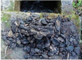
Left, the waterjetter slowly but surely attacked the blockage in the drainline, ultimately opening what had been a badly clogged pipe. Above, the crew extracted numerous chunks of hardened sediment from the pipe.
