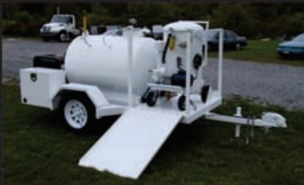
Grease Trap Service Units
