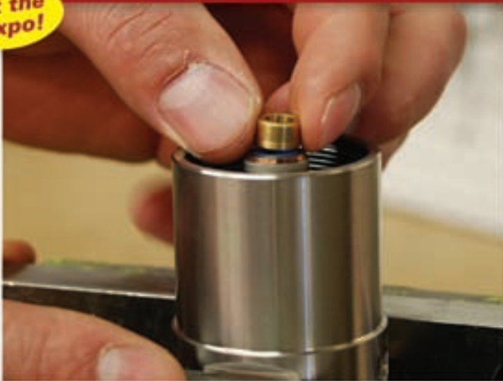
High pressure seats & seals are replaced easily on all Warthog® models.
