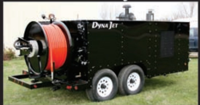
Sewer Jetting Equipment
