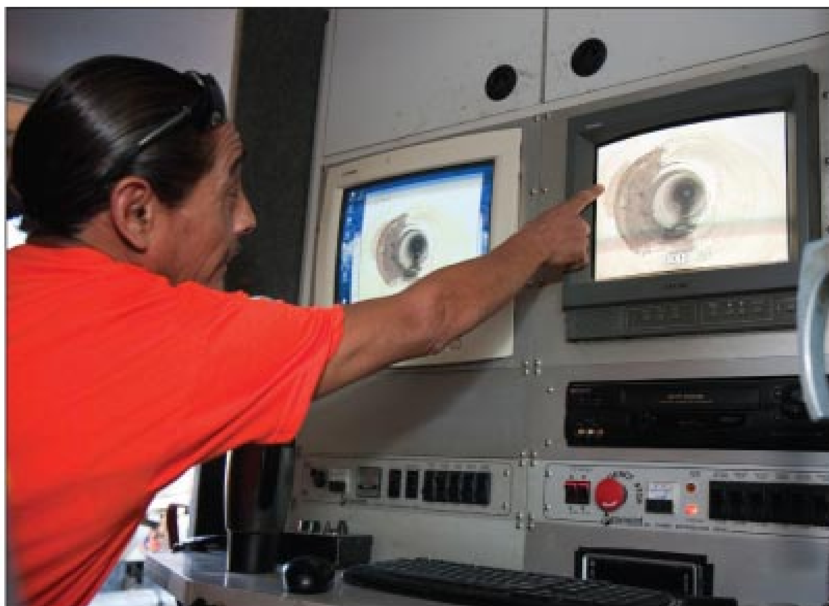
Upper photo: Everardo Canela pulls the hose slowly back to the truck, spreading the herbicide that will kill roots inside the pipeline. Lower photo: Inspection operator Leonard Josytewa watches video as foreman Mark Lei (not shown) lowers a chain cutter into a line.
