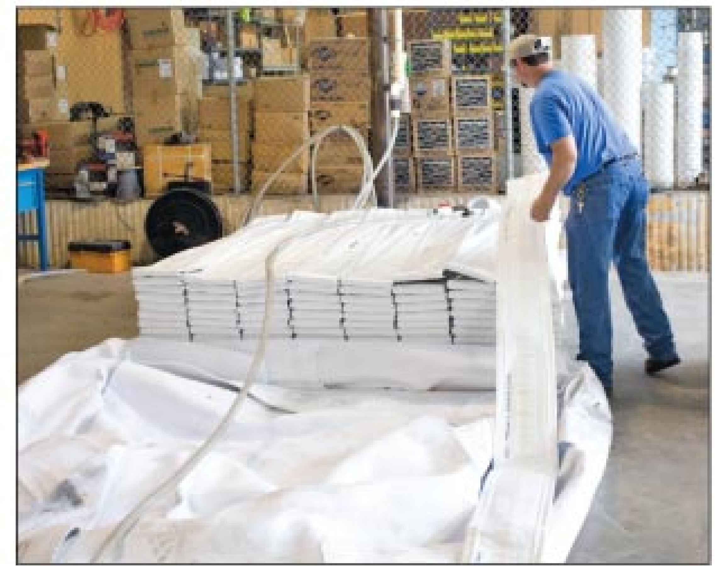
Left: Pipe lining material is prepared in a wet out facility at the Suncoast headquarters. Right: Technician Shay Goff unpacks pipe liner to be coated with resin.
