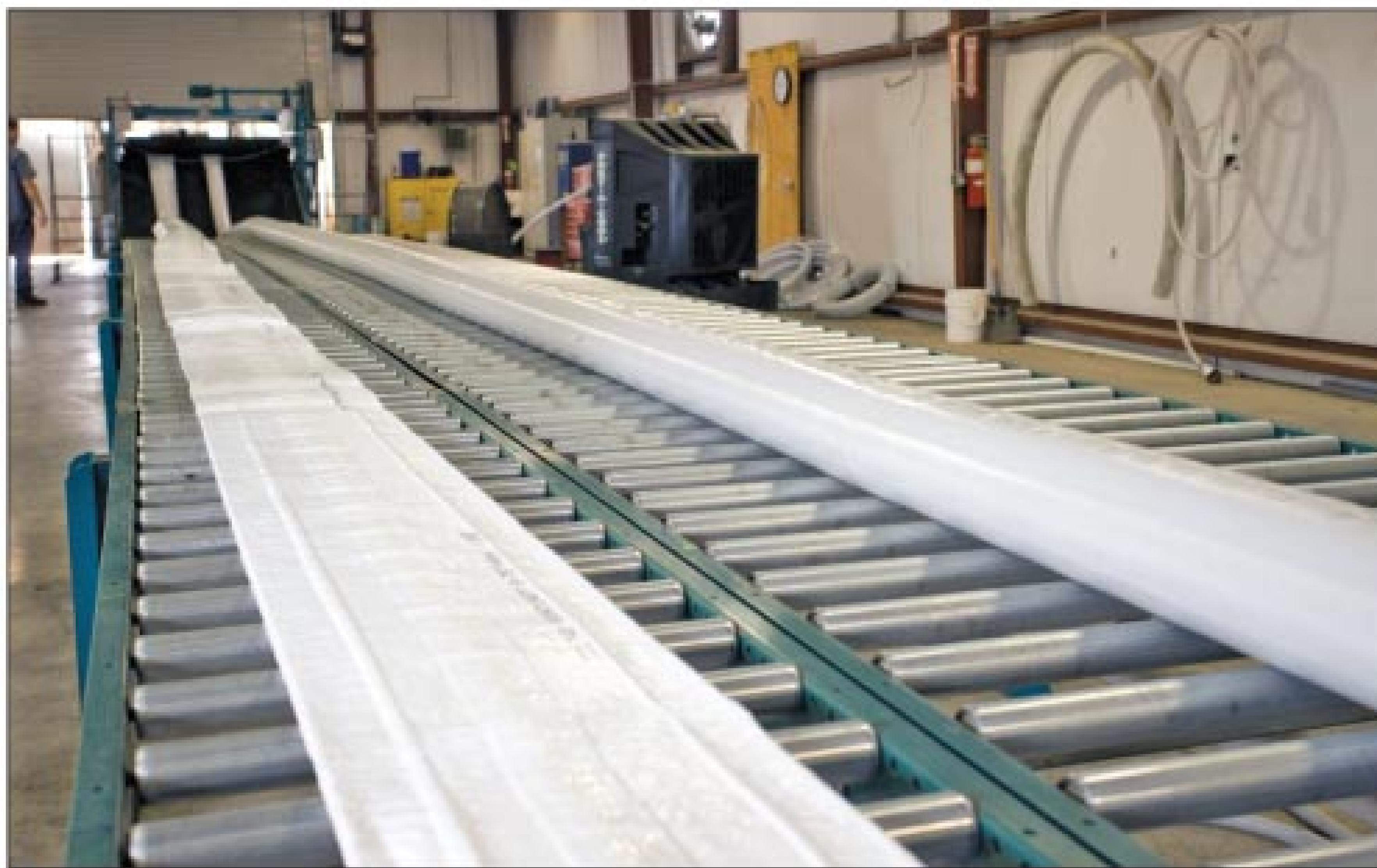
Left: Pipe lining material is prepared in a wet out facility at the Suncoast headquarters. Right: Technician Shay Goff unpacks pipe liner to be coated with resin.
