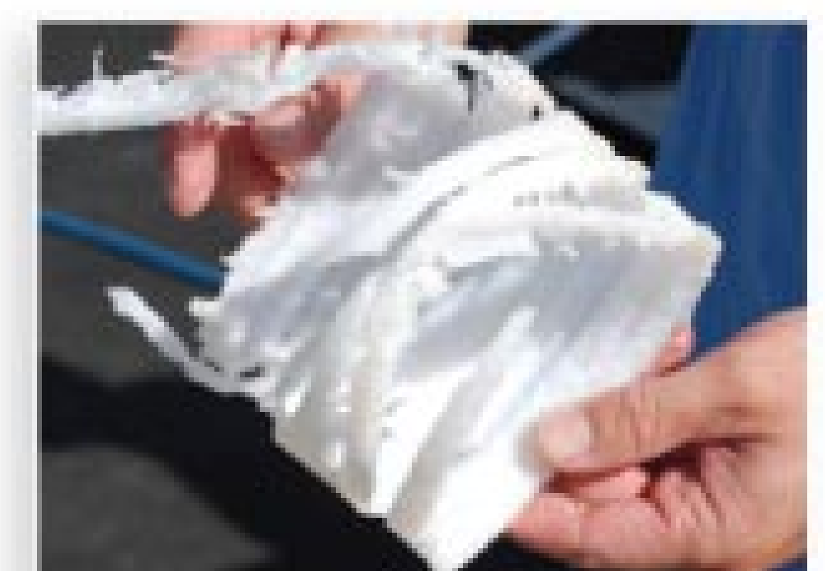
UHMW-PE plug destroyed.
