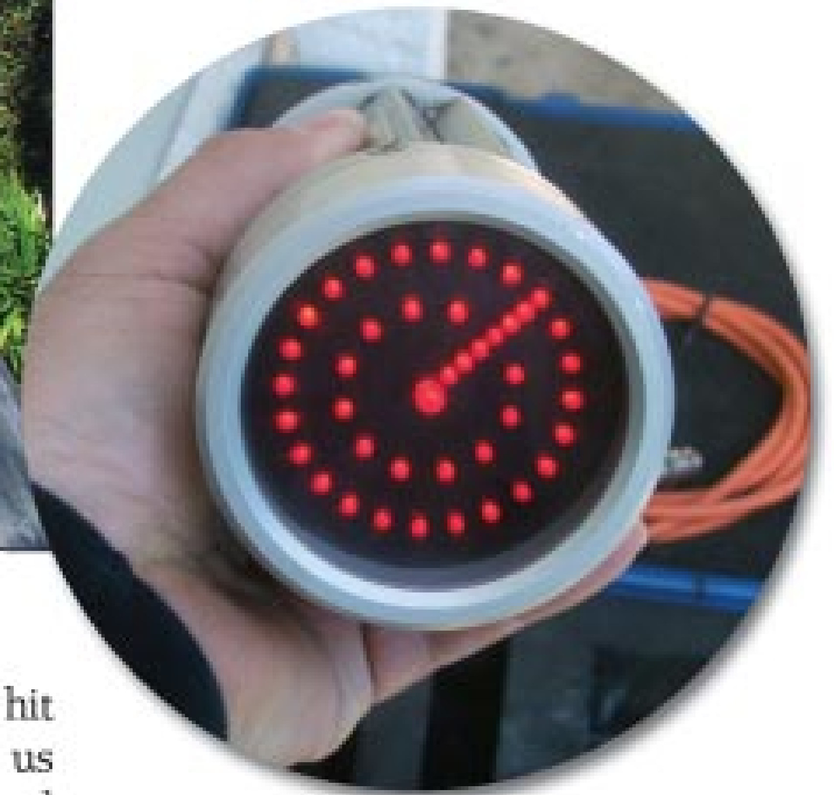
The LED target is mounted behind the boring head. The camera can see it through the hollow rods.
