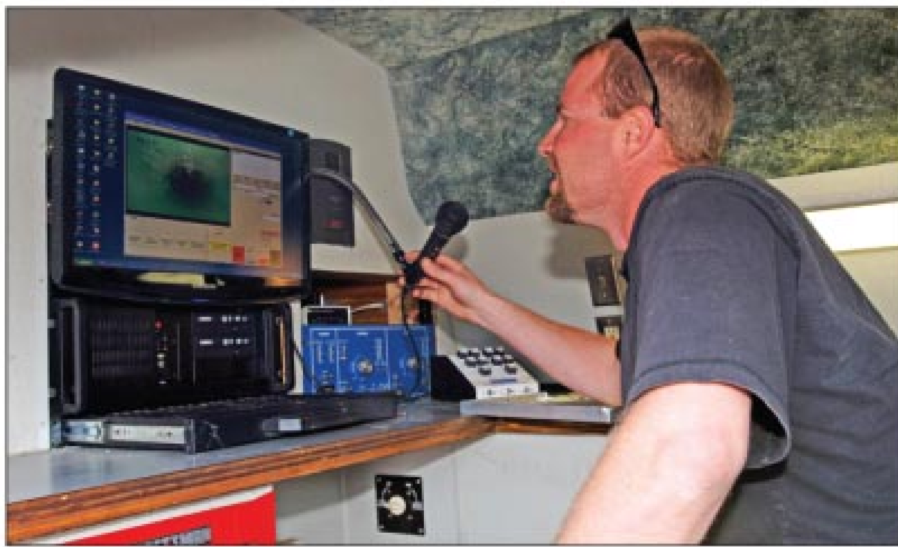
Titus Larsson conducts video inspection with an OmniEYE III tractor-mounted camera from RS Technical Services.
