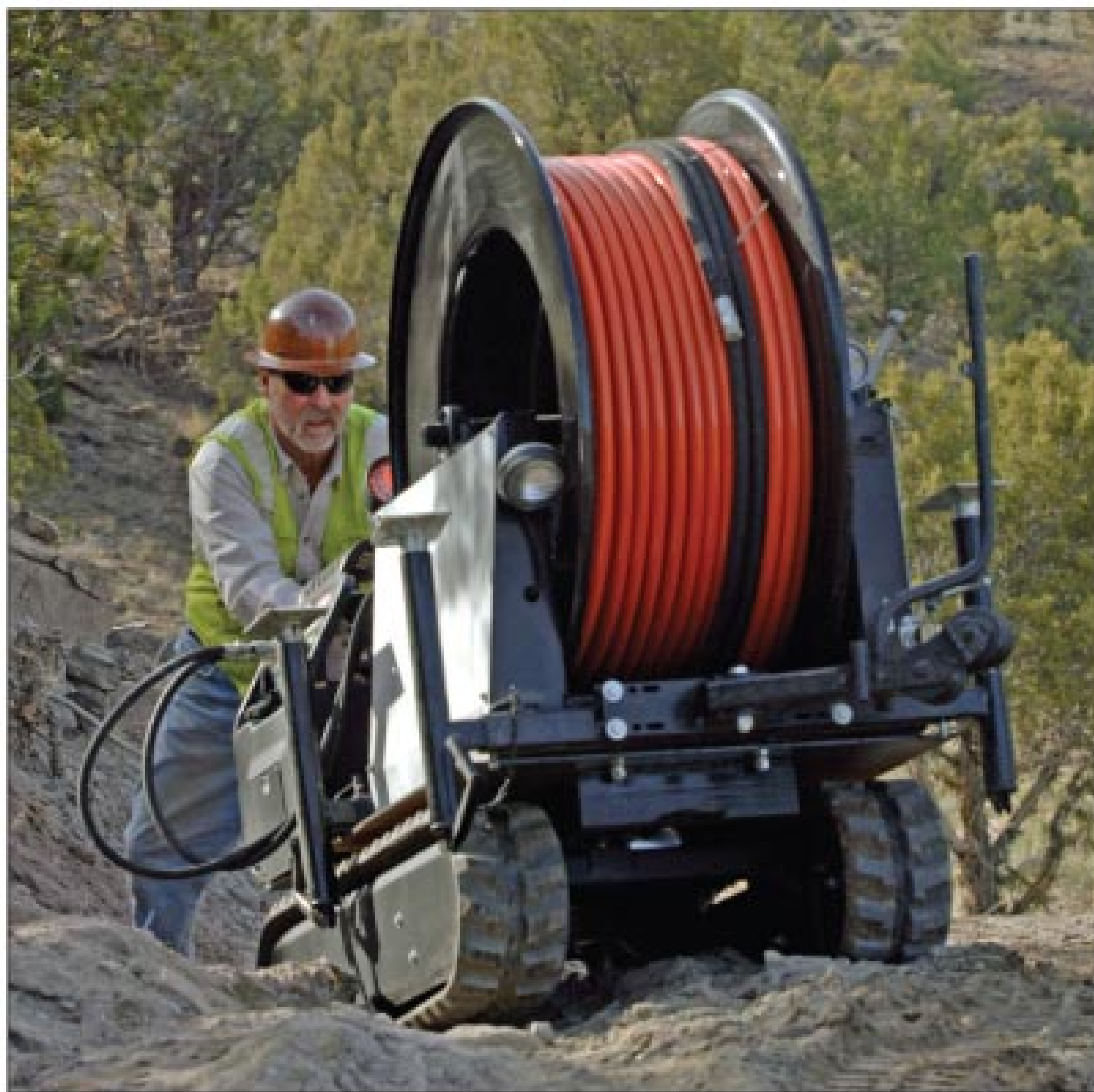
Left photo, Bob Rasnick moves an easement jetter made by Jack Doheny Supplies to an off-road work site. Right photo, Titus Larsson feeds vacuum tube into blocked culvert.
