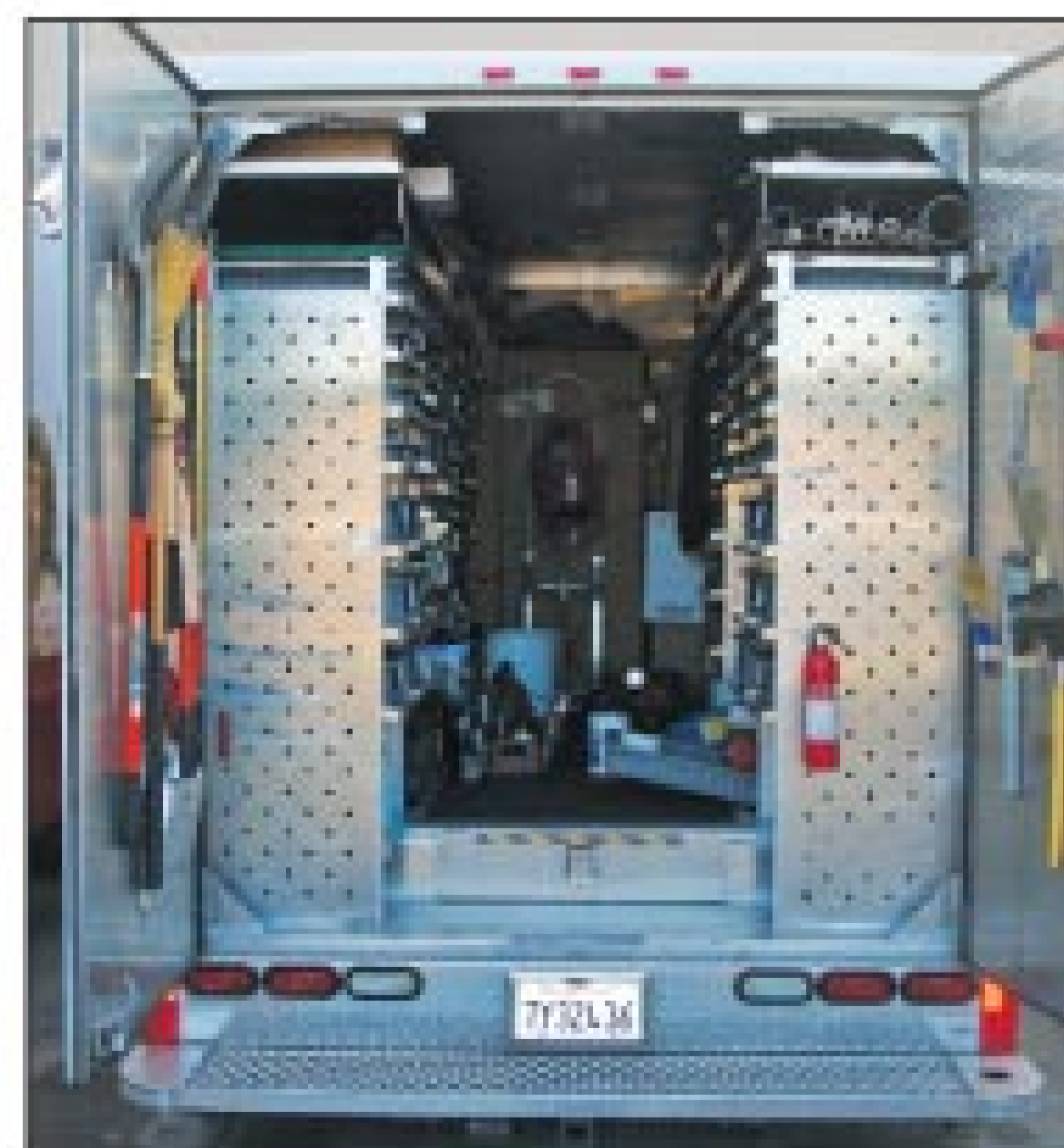
All service trucks are set up identically with numbered bins assigned to specific parts and supply items.
