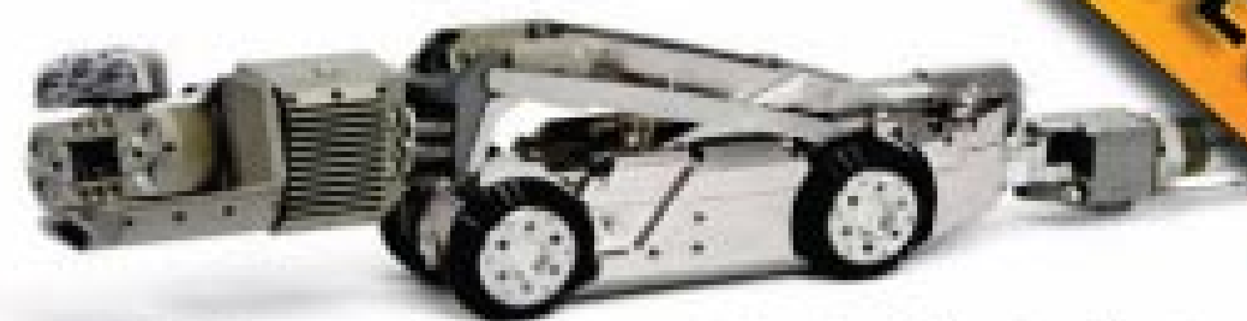
L135 Tractor with the Laser Pipe Profiler Application
