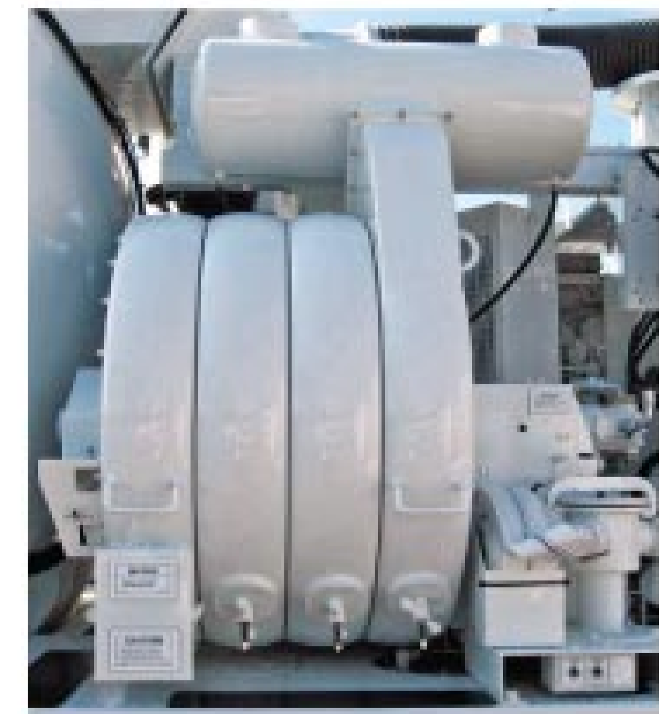
Vac-Con Inc.: Three-stage fan vacuum system
