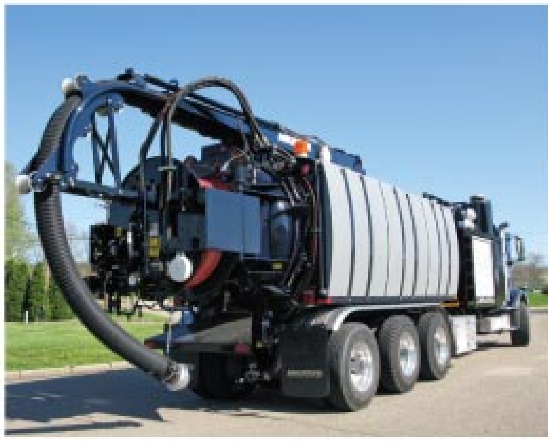
Hi-Vac Corp.: Rear hose reel design
