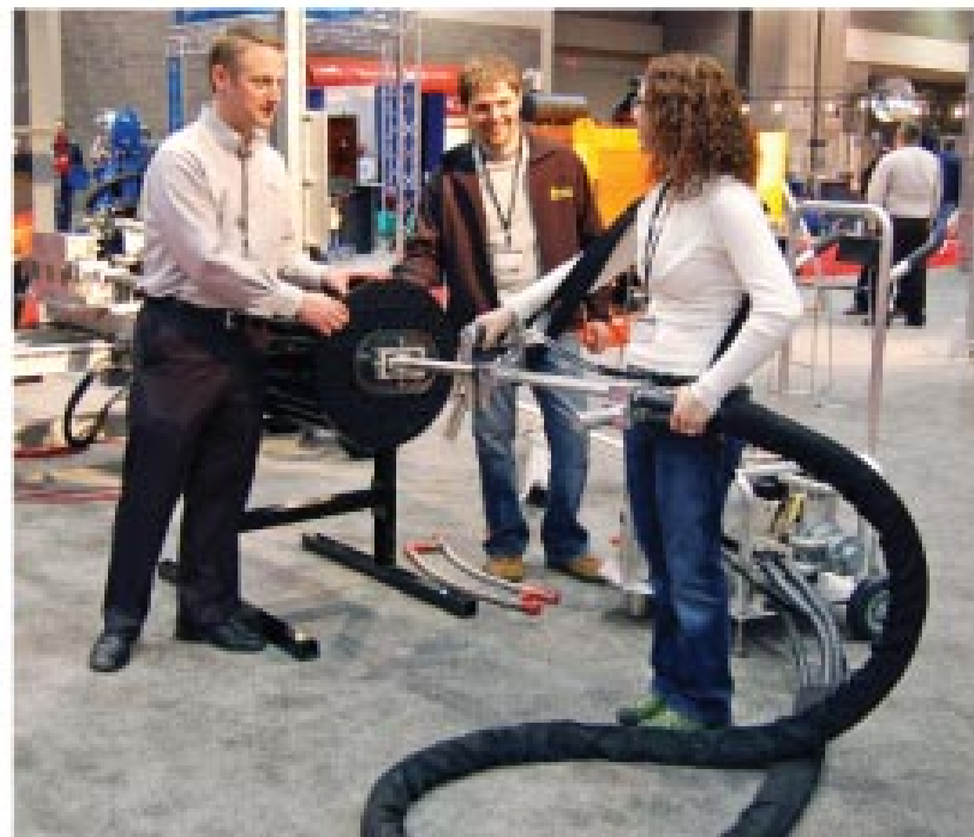
Saflex-2000 semi-automated tube lancing system from NLB Corp.
