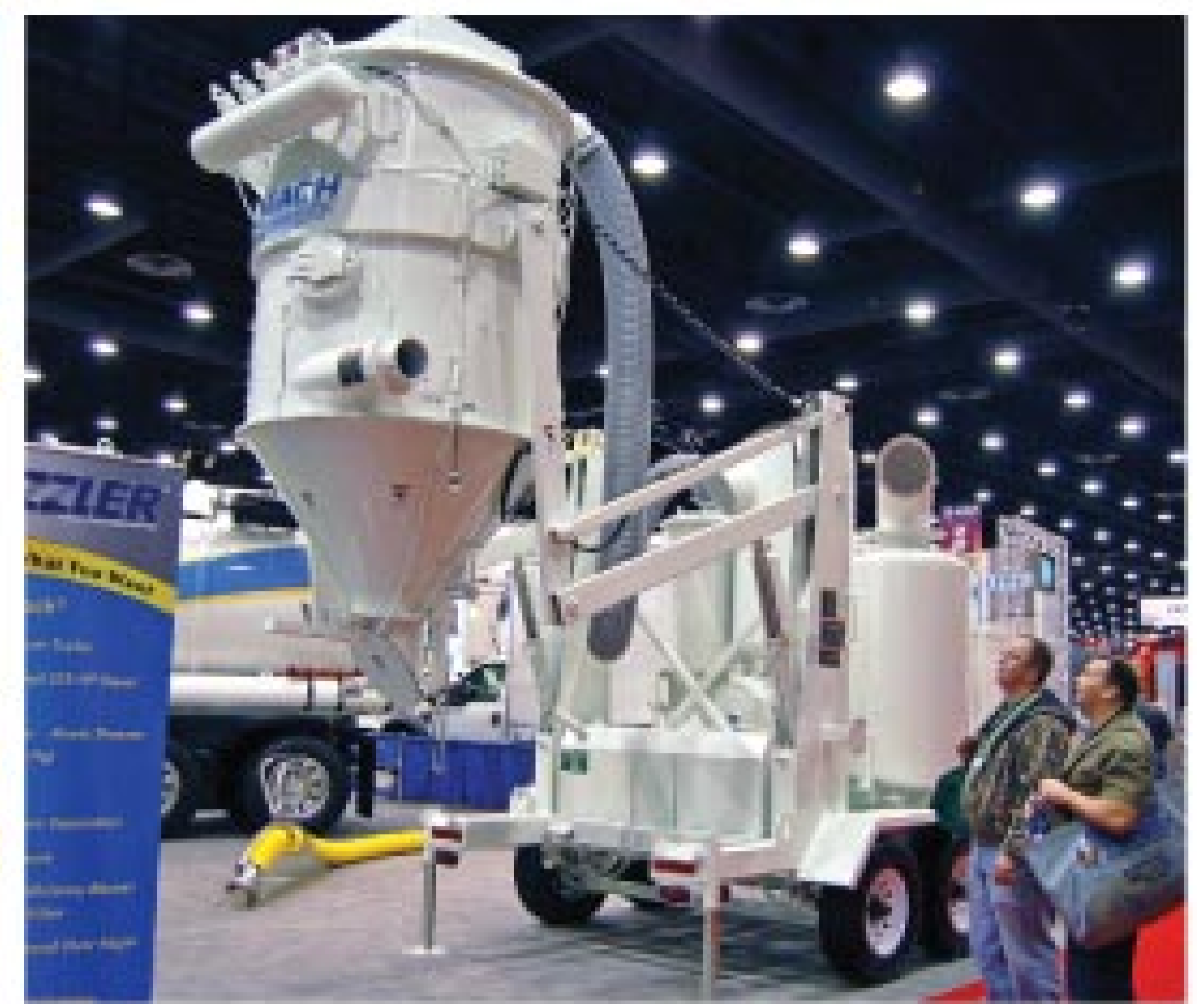
Reach trailer-mounted vacuum system from Guzzler Manufacturing.
