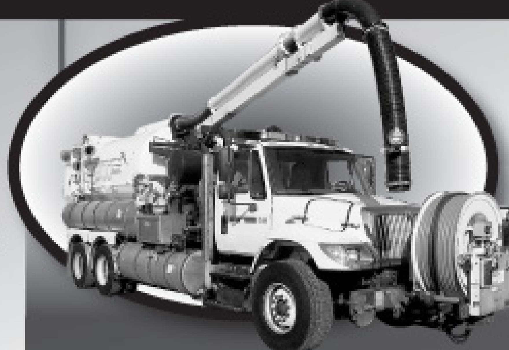
2003 INTERNATIONAL 7400 ; 10 Yard Debris Tank W/Pump Off, Vactor Pump 80 GPM @ 2500 PSI
