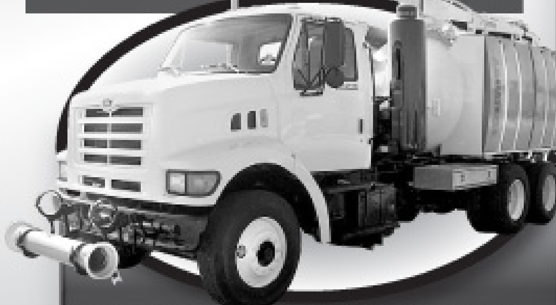
1997 FORD LOUISVILLE 1997 AQUA-TECH B-10 , General Pump 83.5 GPM @ 2000 PSI, Roots 624 Blower, Hydraulic Rear Open Door And Locks.
