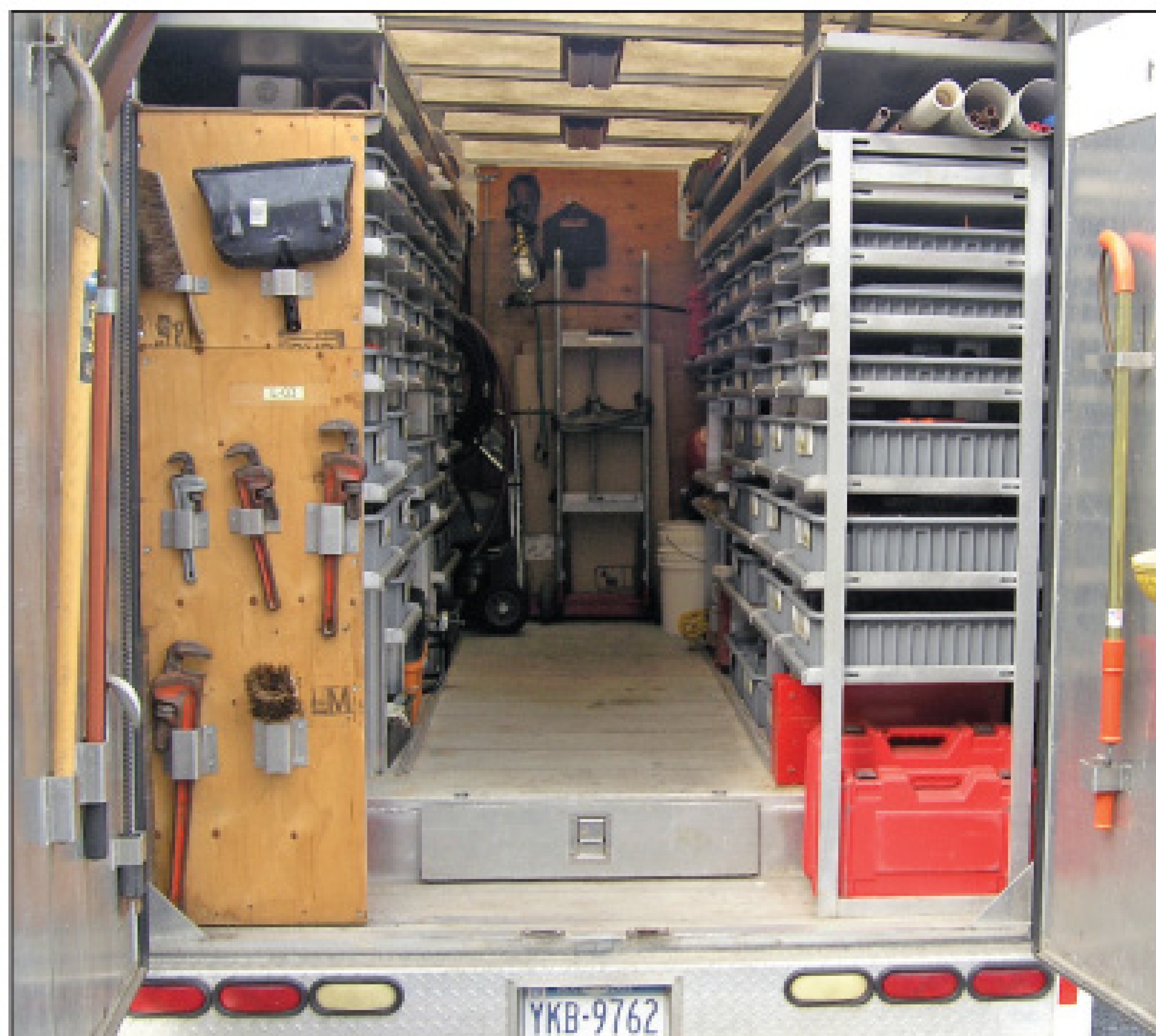
The 2002 Isuzu NPR truck carries a Hackney P2000 plumbing service body. Inside, the adjustable-shelf storage system holds 75 plastic bins, each labeled with a letter and numbers to simplify part location.
