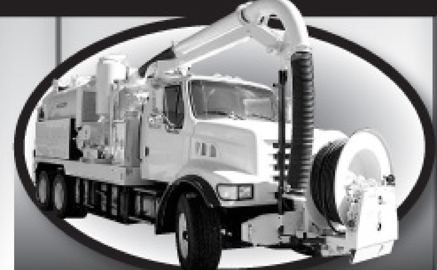
1998 FORD LOUISVILLE ; 1998 Vac-Con, Vac-Con Plunger Pump 50 GPM @ 3000 PSI, Roots 827 Blower, 12 Yard Debris Tank, 3/4" Jetting Hose, John Deere Pony Motor, 4872 Hrs.
