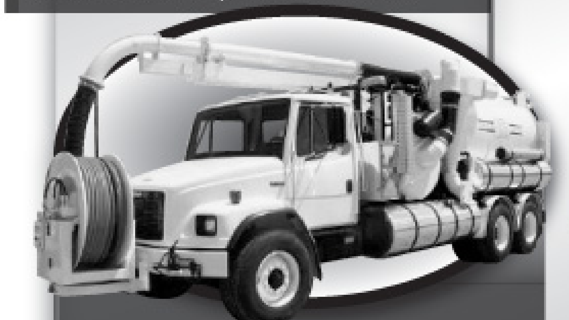
1998 Freightliner FL-80 VACTOR : 2110-06 S/N: 97-05-6161 Vactor Pump 80 GPM @ 2500 PSI 1
