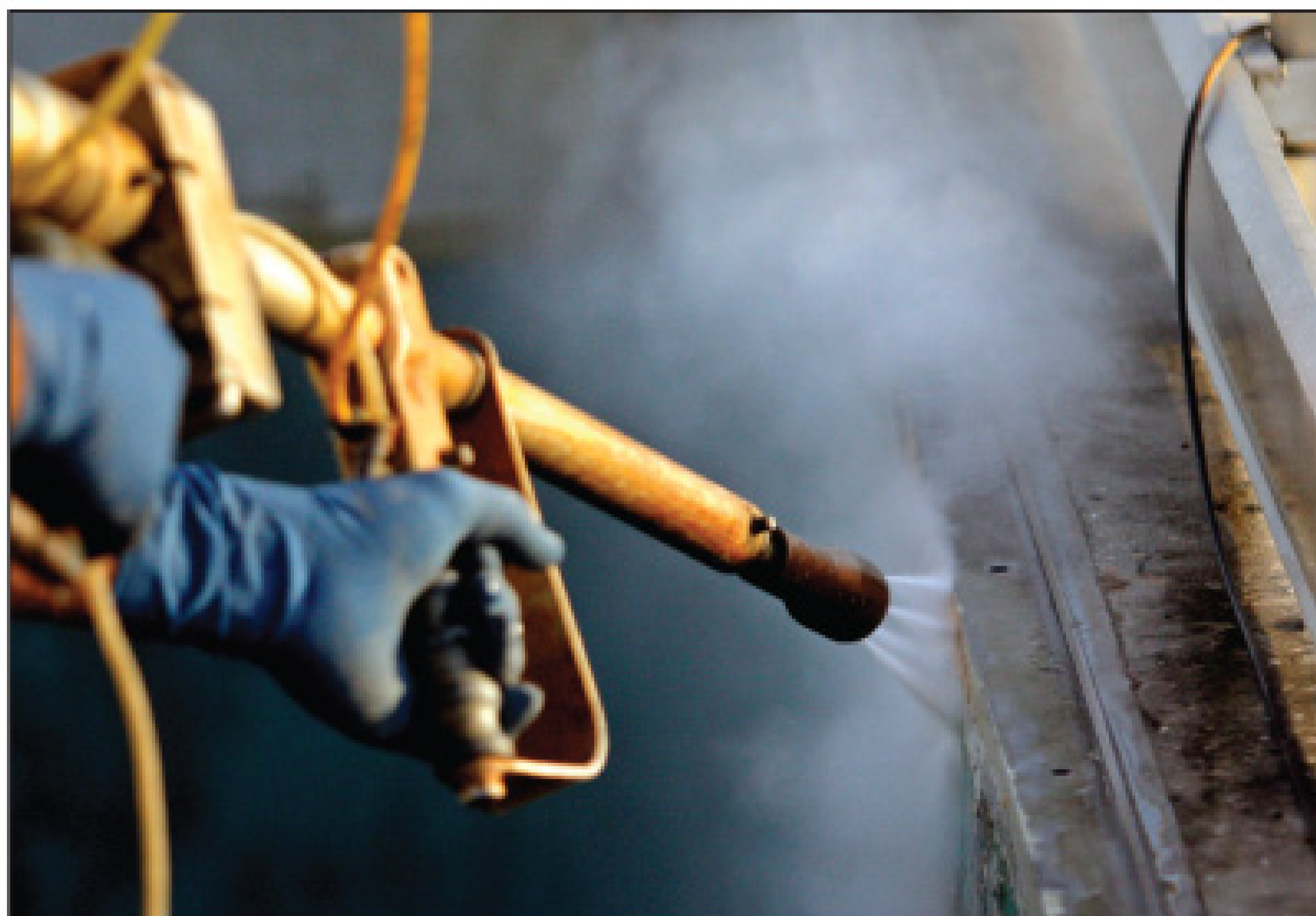
The company's Aqua-Miser can deliver water at 40,000 psi to ensure a completely cleaned surface, ready for recoating.
