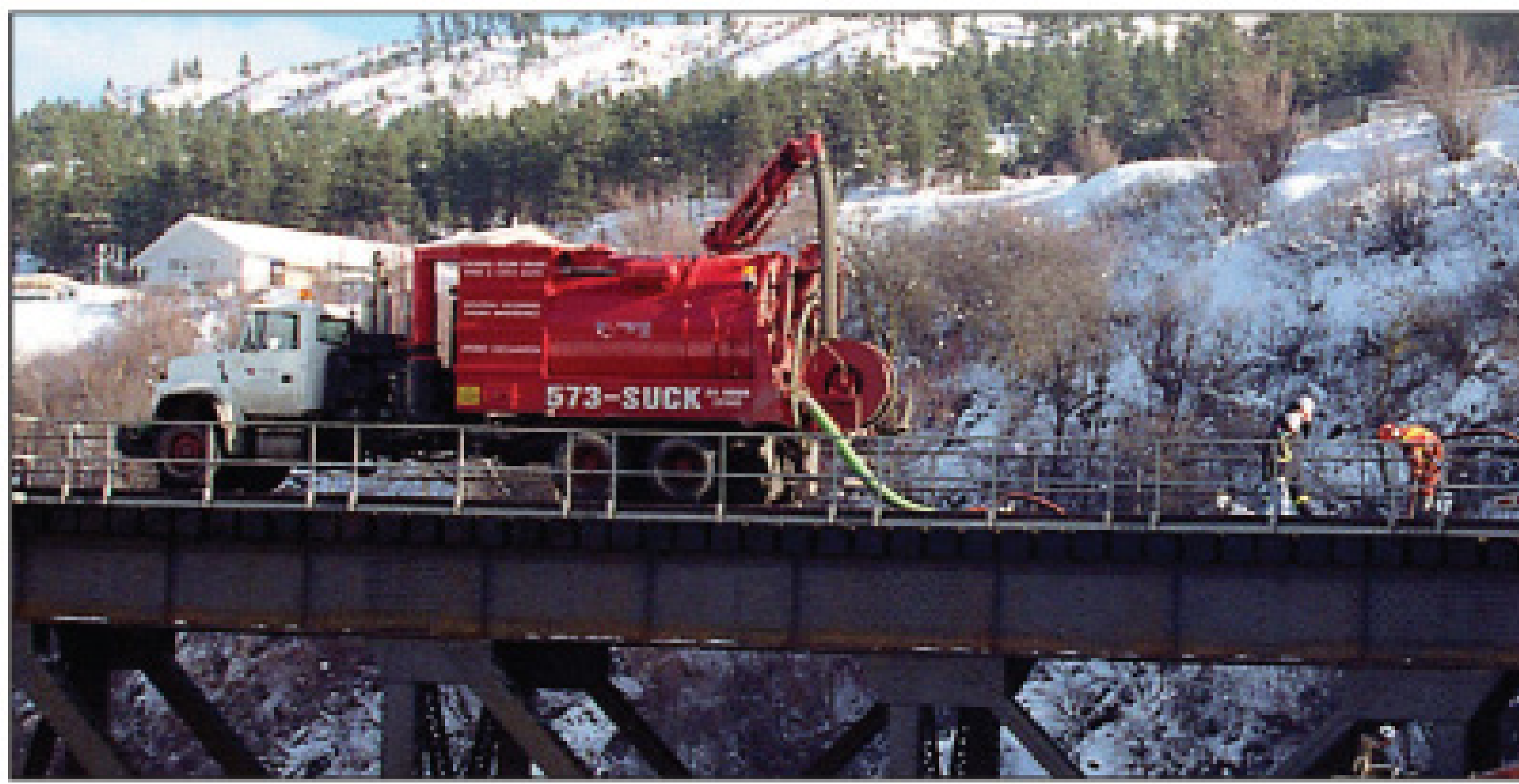
A rail package enables the vacuum truck to get to railroad spills quickly and easily for clean-ups.
