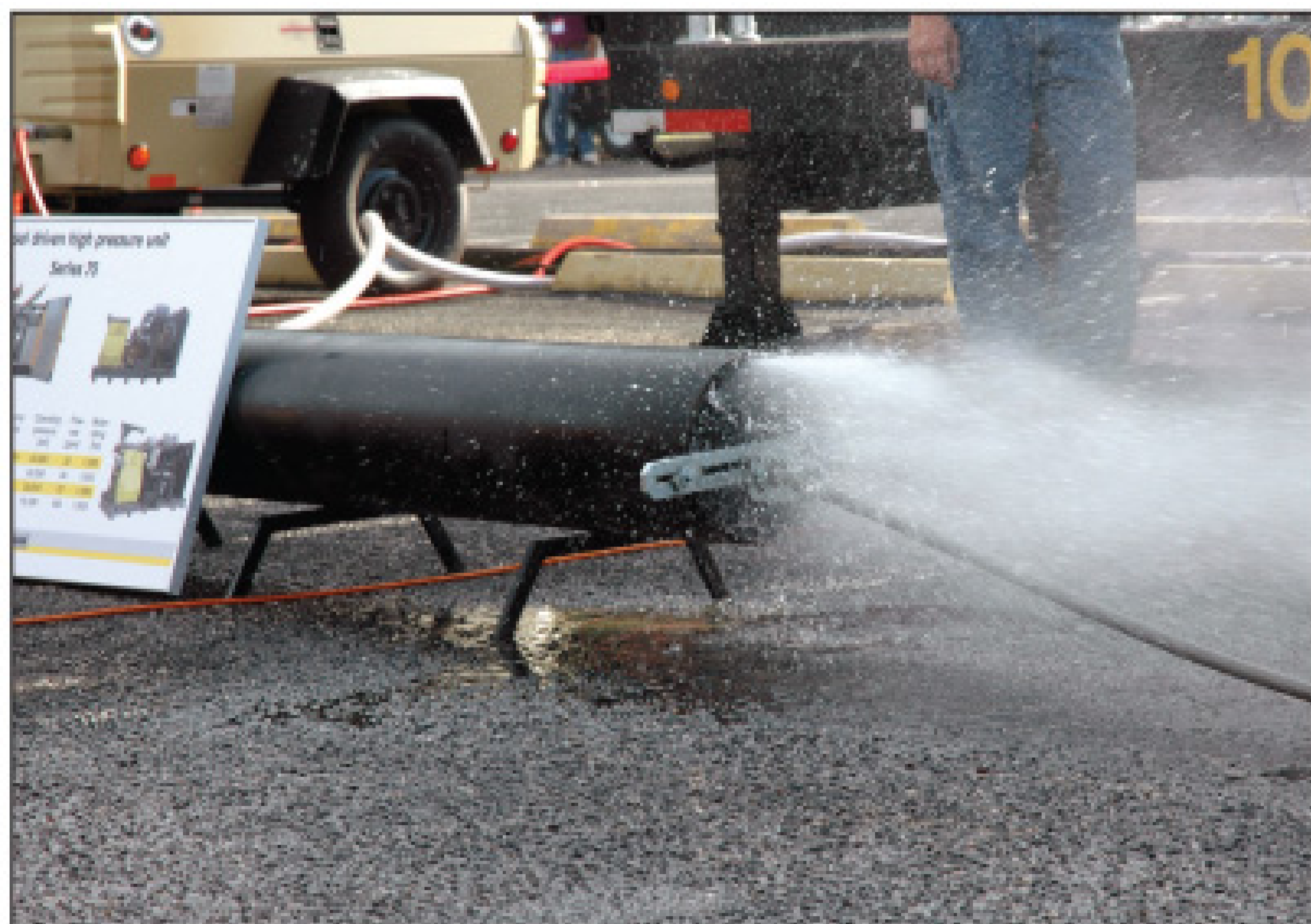
Hammelmann Corp. demonstrated its 1,000 hp pump and 3D reaction-force-driven internal pipe cleaning device at the 2009 WJTA conference.
