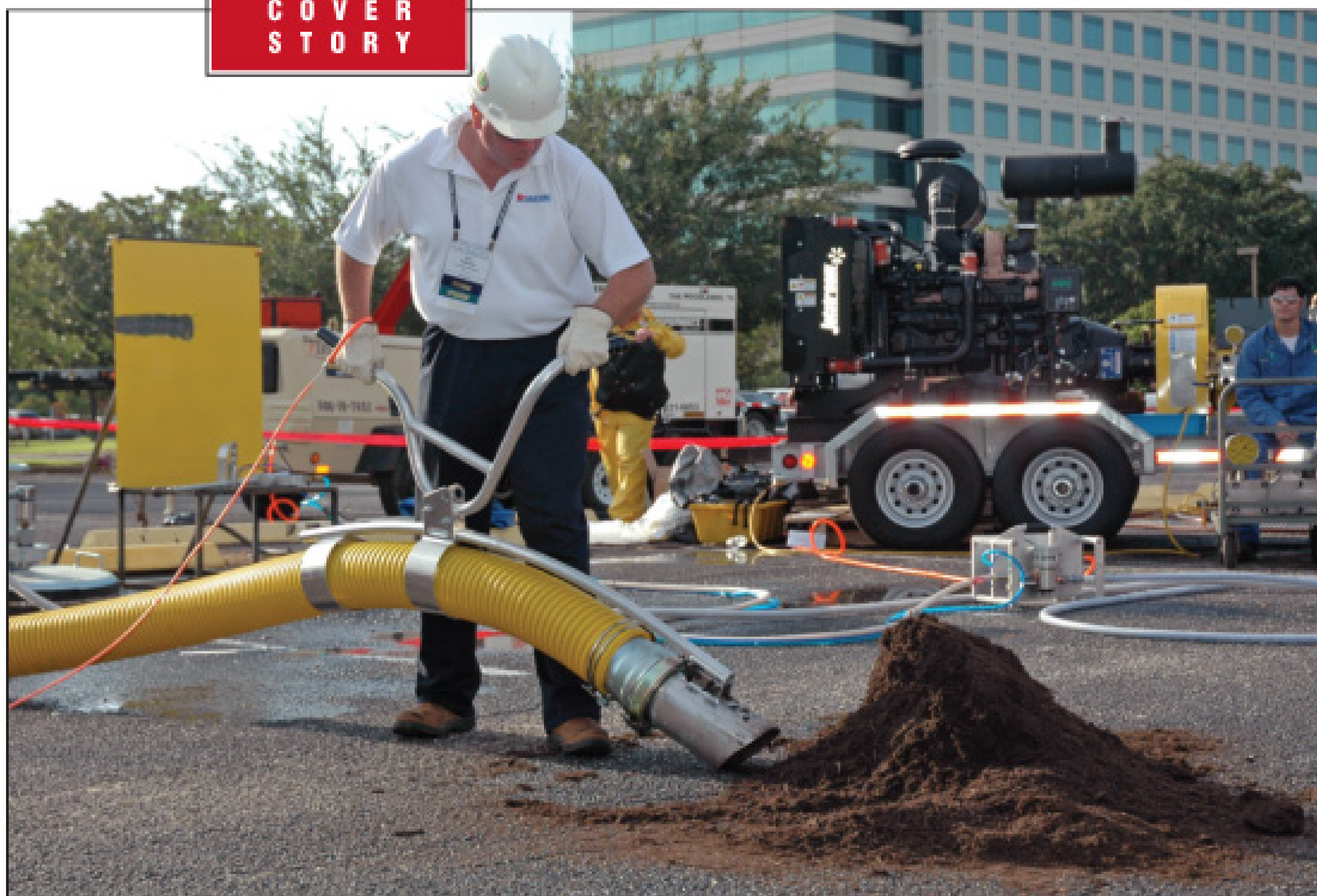
Don Calhoun of Guzzler Manufacturing Inc., demonstrates the use of GuzzlerGrip nozzles for industrial vacuuming applications at the 2009 WJTA exposition.
