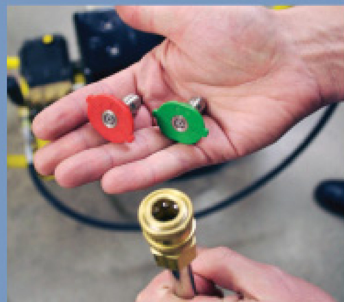
Basic maintenance on a pressure washer includes, clockwise from the top left, changing the tips, changing the oil, checking the tip size, and changing the filter.
