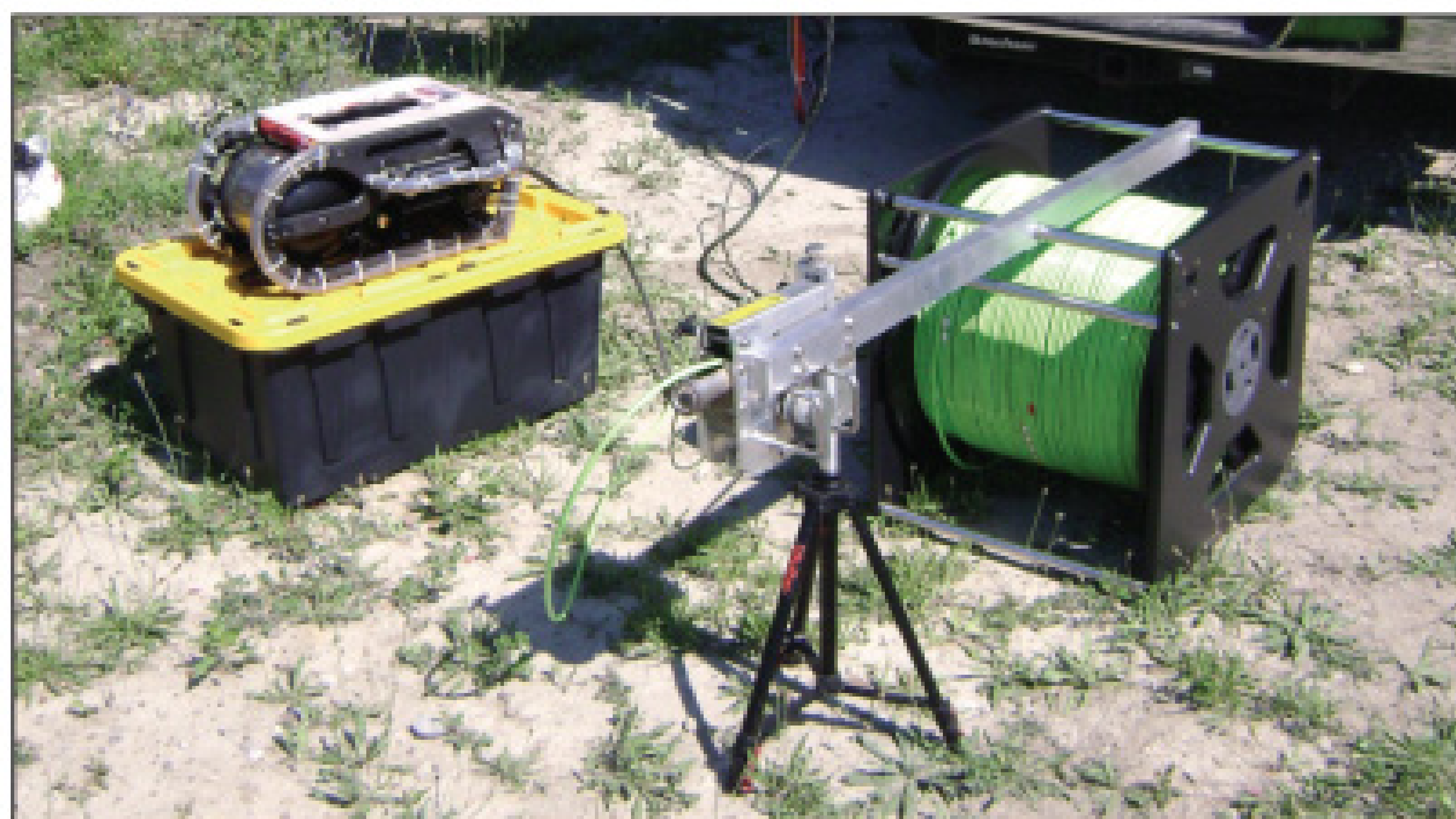
The SeaBotix LBV300XL is ready to inspect the intake pipe after the pipe was cleaned.
