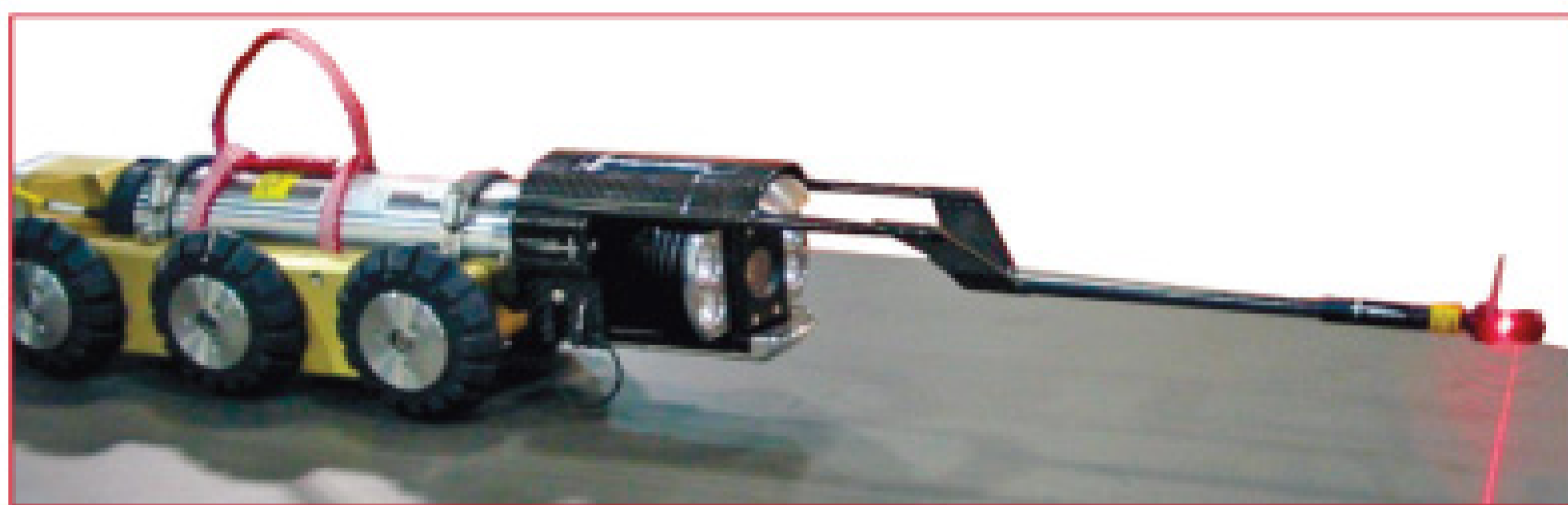
In this common laser profiling configuration, a CUES LP917 laser profiler is shown coupled with an OZII video camera.
