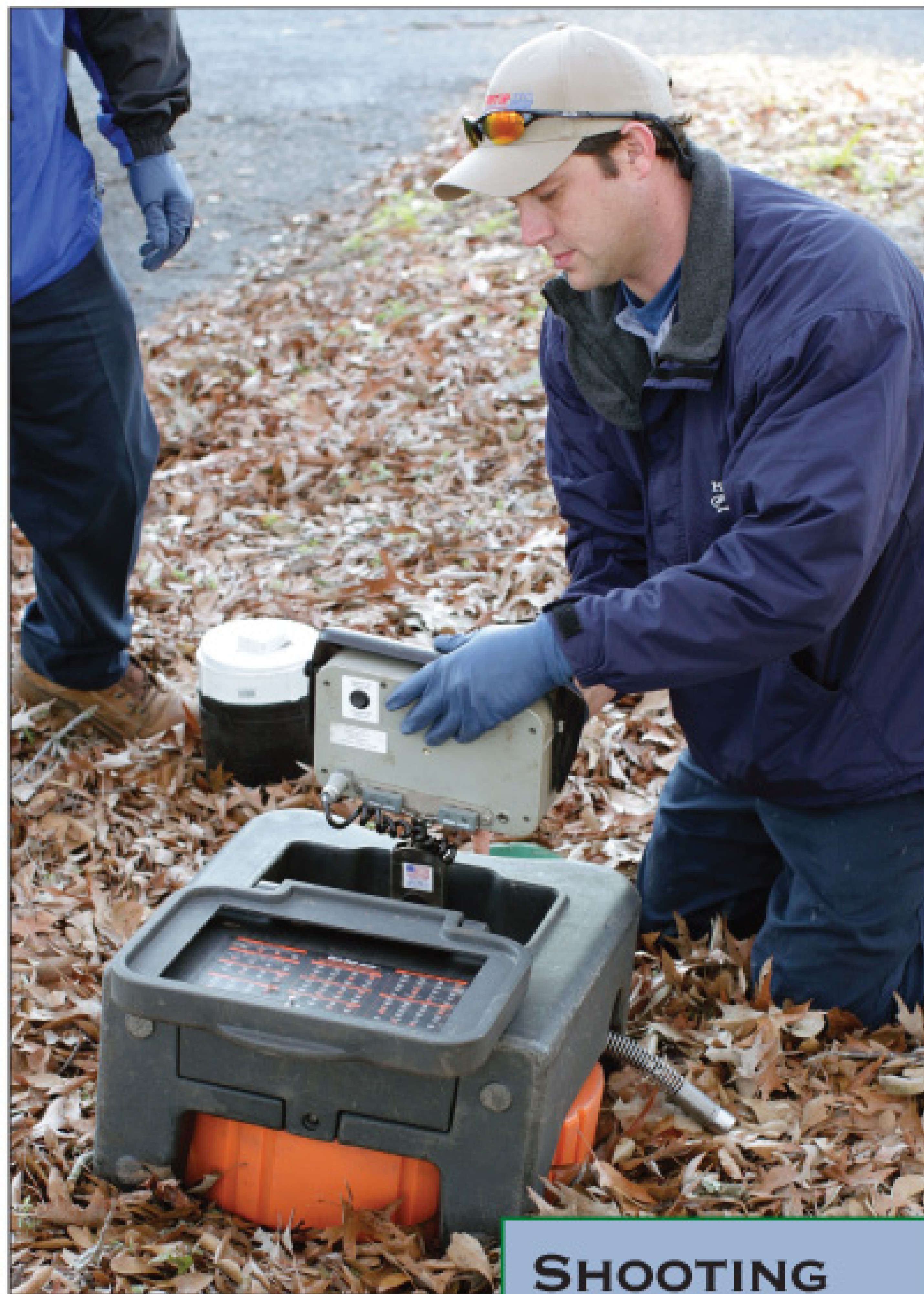
Greider uses one of the company's inspection tools, a Gen-Eye Junior camera from General Pipe Cleaners.
