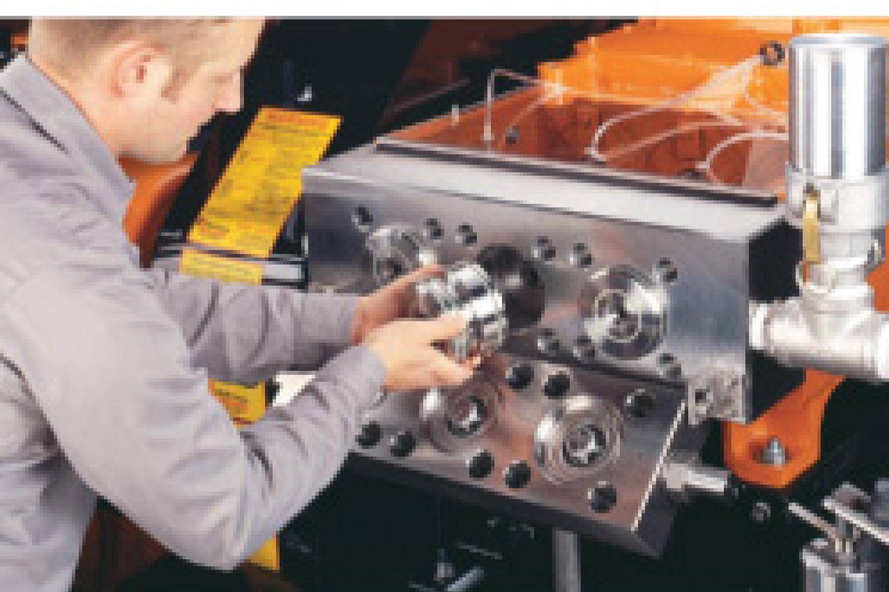
Convert the NLB 225 to 40,000 psi in just 30 minutes — 20 minutes for lower pressures.
