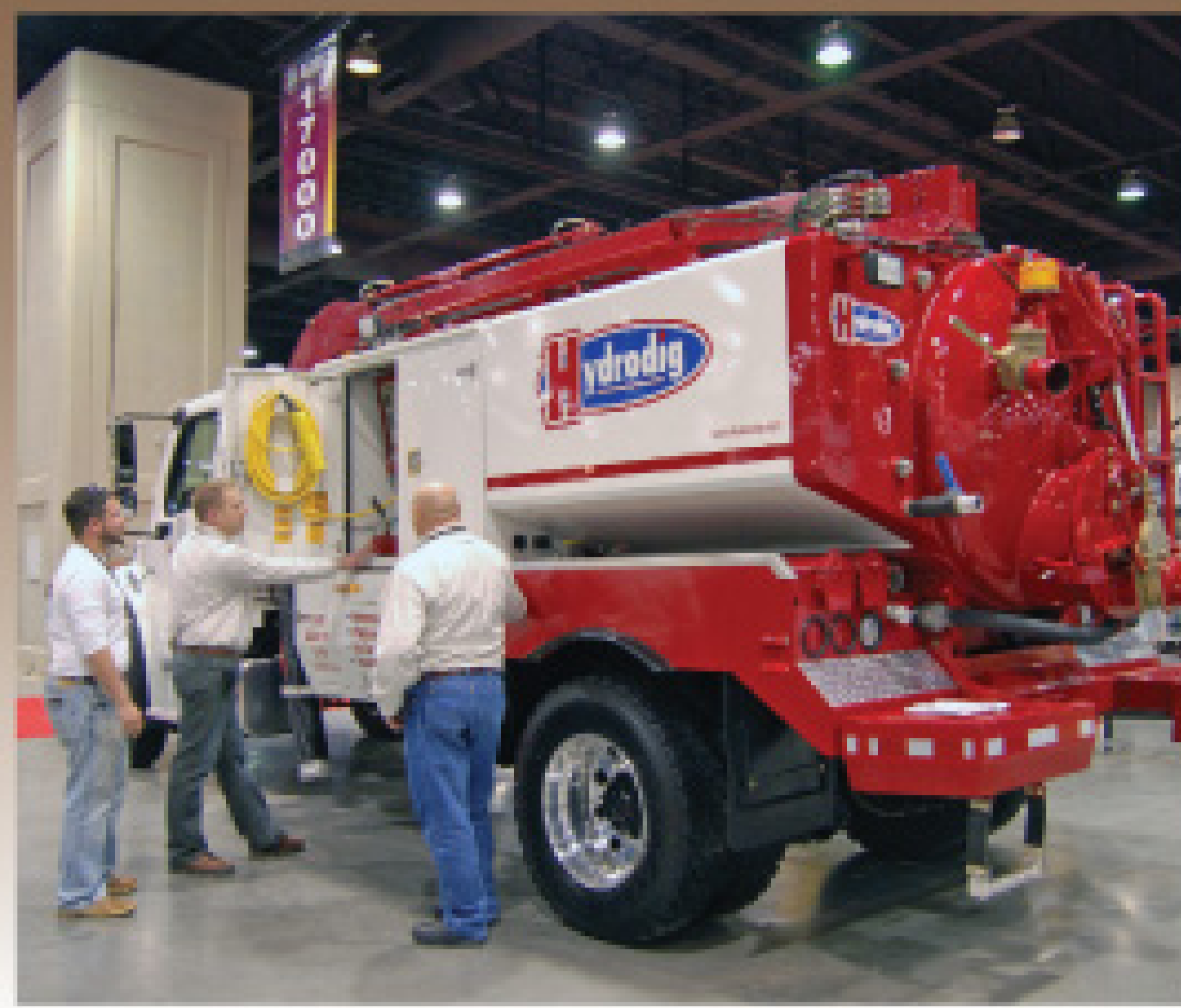
Hydrodig vacuum excavator from Hydrodig USA LLC.
