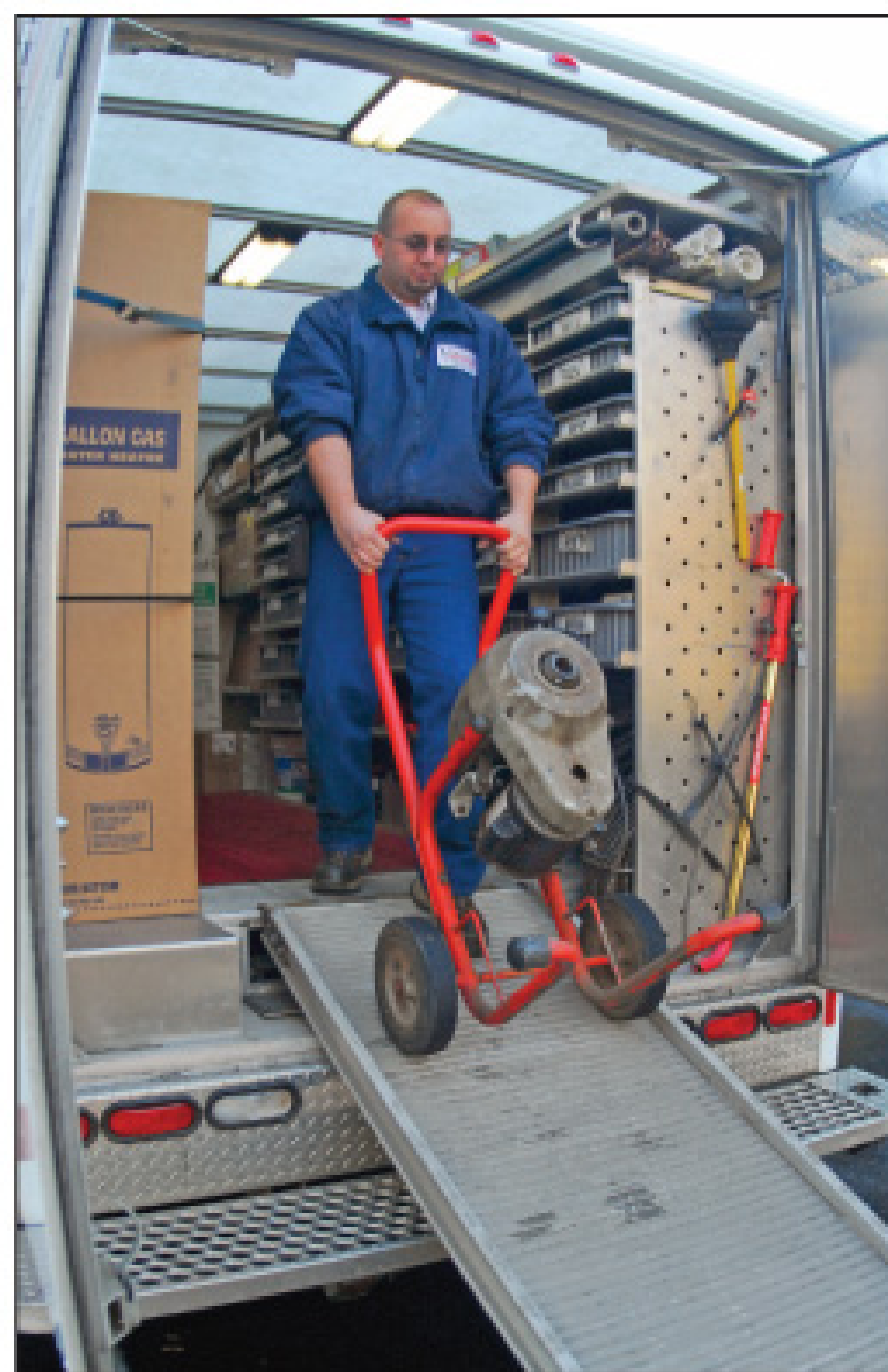
The custom-made parts storage system (right) includes coded bins, so that, for example, part number L1206 is located on the left side of the truck, bin 12, slot 6.
