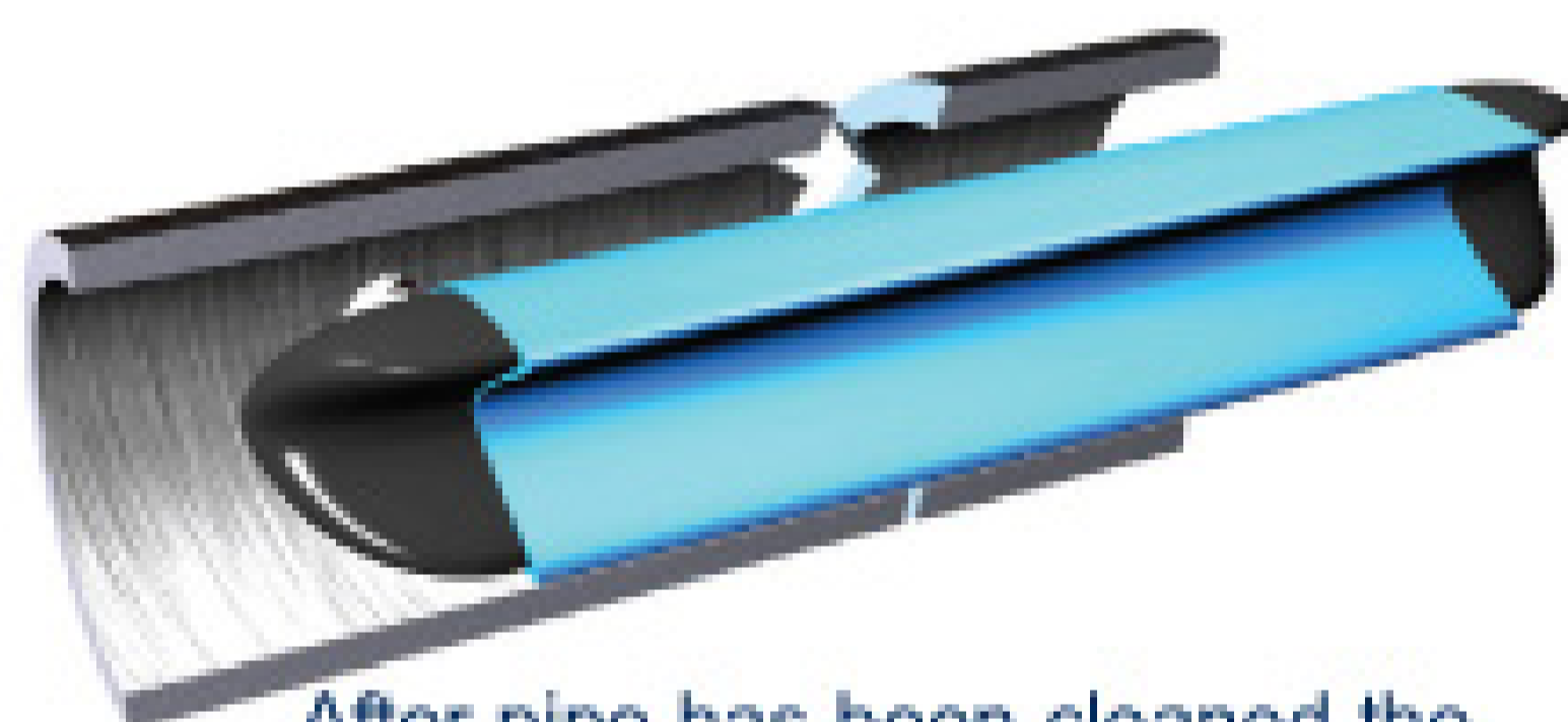
After pipe has been cleaned the liner is pulled-in-place and inflated
