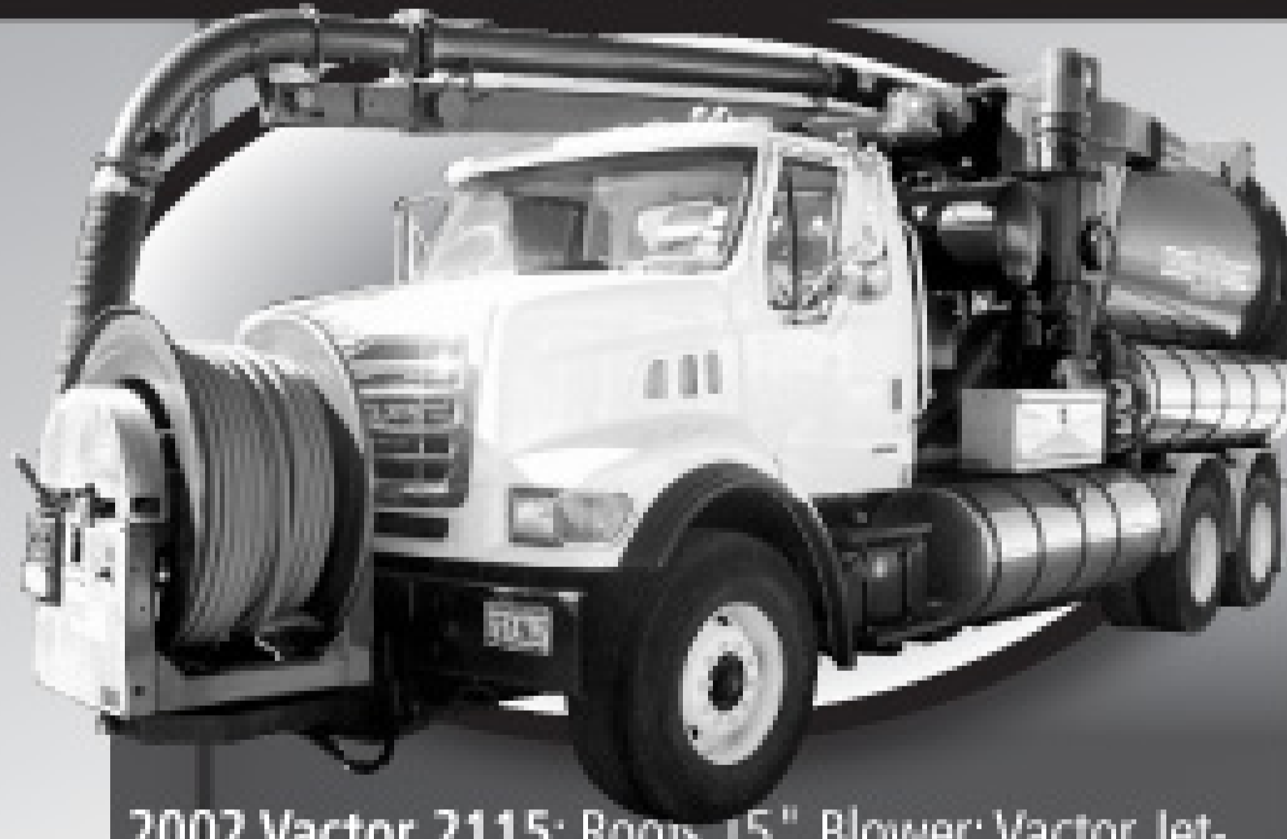
2002 Vector 2115; Roots 15" Blower; Vector Jetting Pump 80 GPM @ 2000 PSI; 15 Yard Debris Tank with Body Flush Out, and Pump Off Systems!
