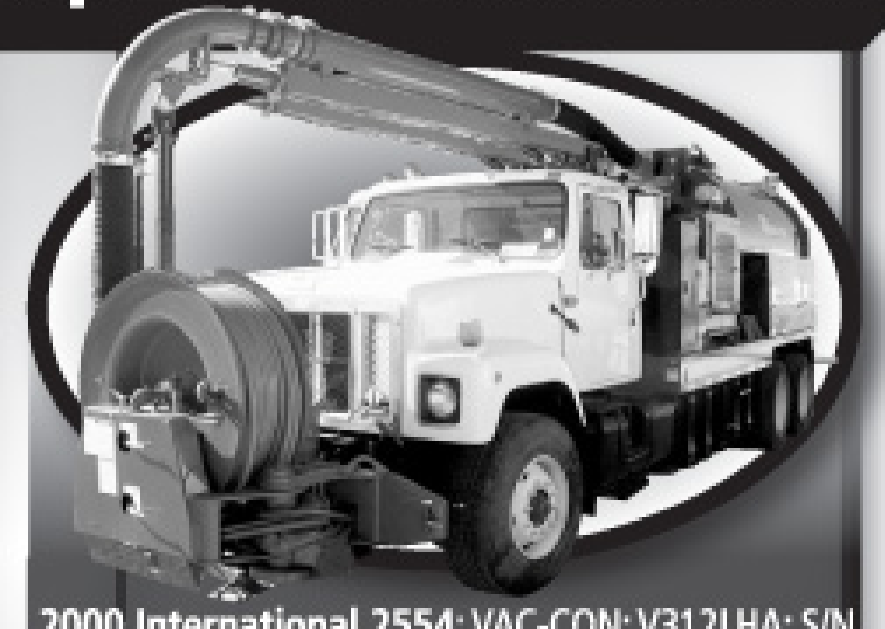
2000 International 2554; VAC-CON: V312LHA; S/M 08992206; 3 Stage Fan Unit; 12 Yard Debris Tank; John Deere Rear Engine; Bean 80 GPM Pump
