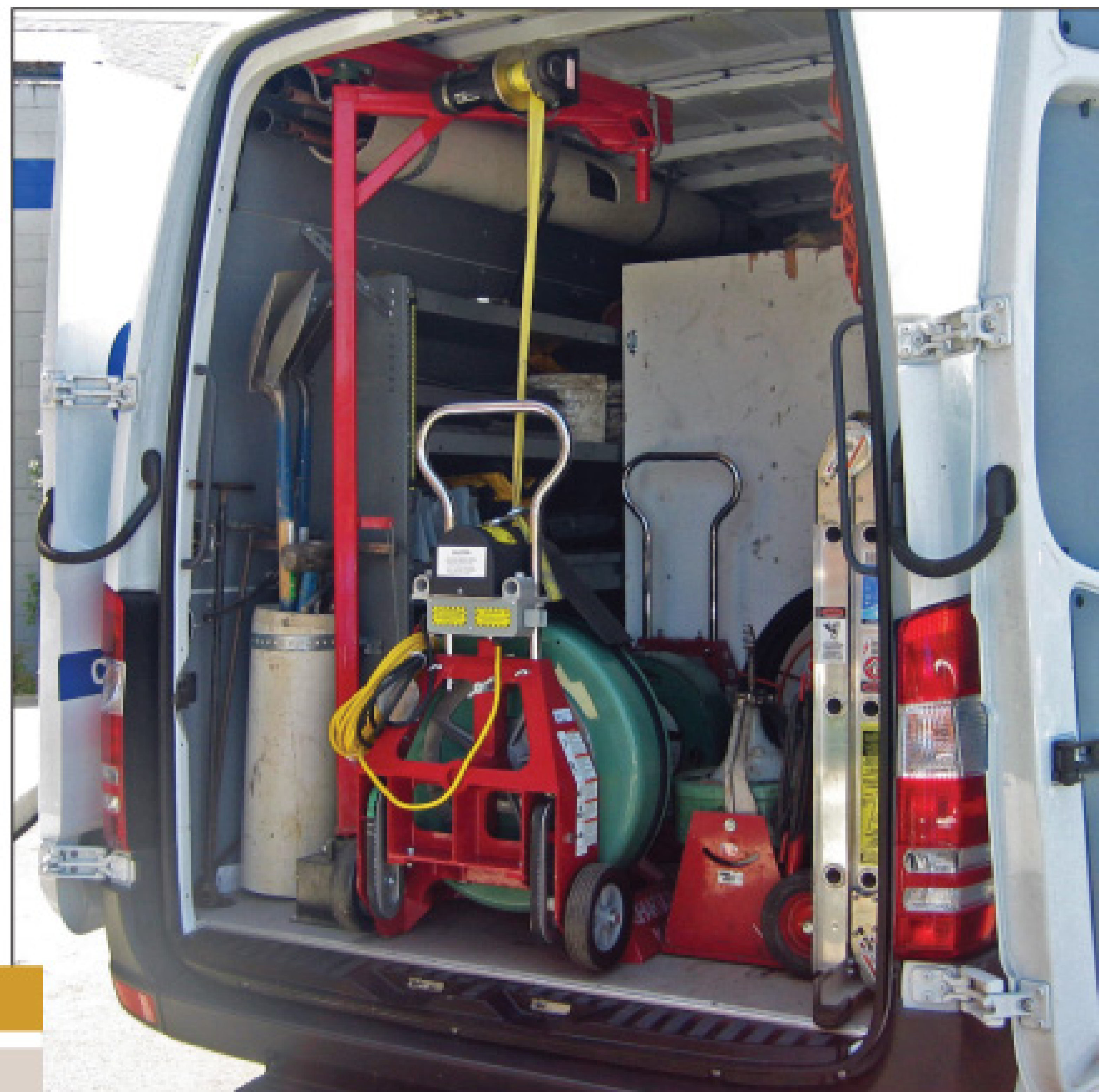
To prevent equipment damage and employee injuries, Frank Bonetti Plumbing of Castro Valley, Calif., has outfitted its service vans with the Vancrane, a rear-mounted, 1,500-pound-capacity electric crane made by Pickup Equipment Inc. (Photos courtesy of Frank Bonetti Plumbing)
