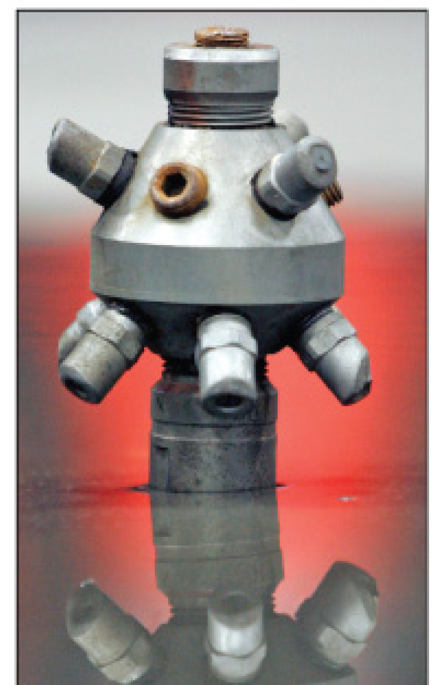
A 20,000-psi cleaning nozzle used by United Industrial Services.
