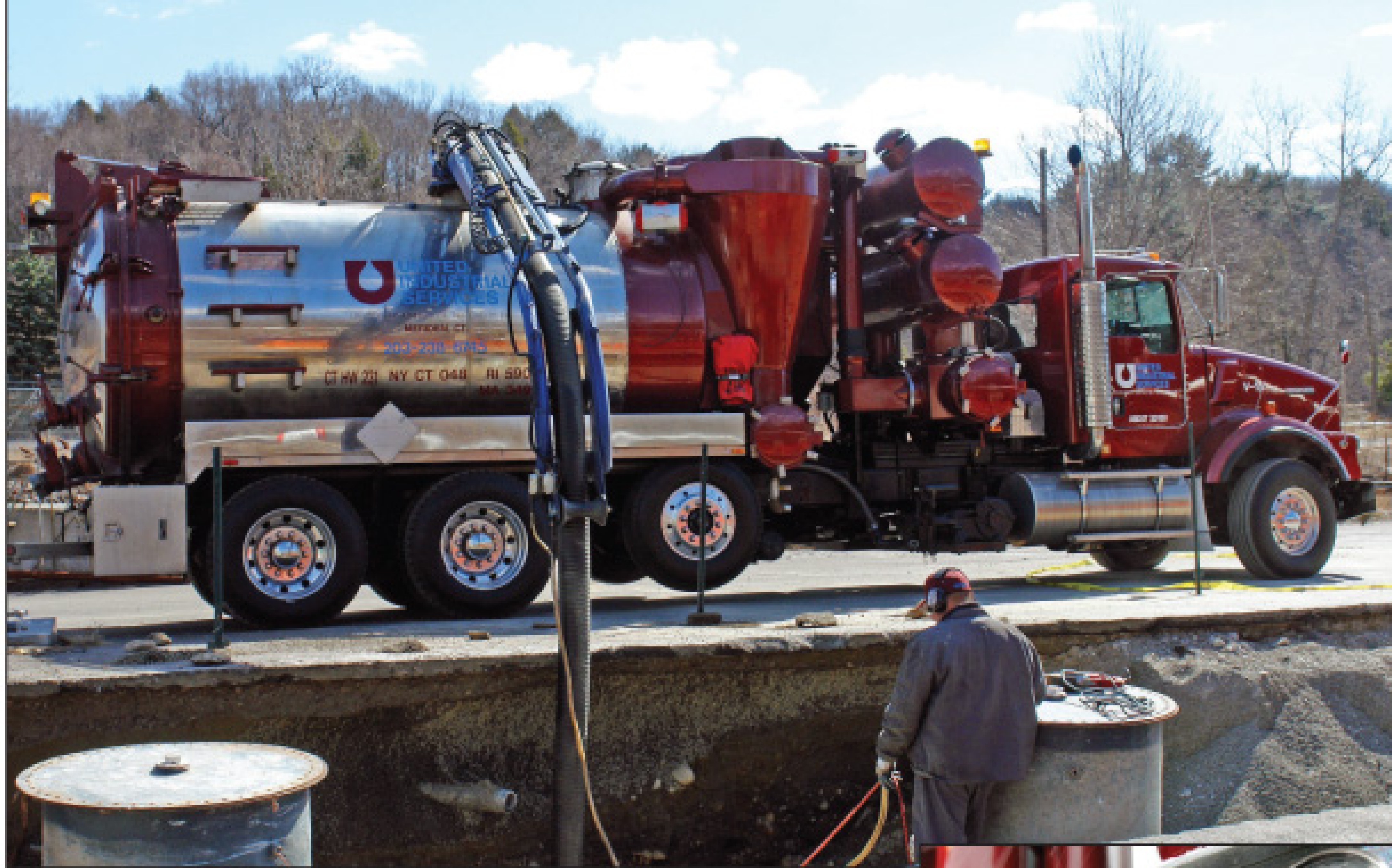
Top: A high-capacity vacuum truck is used to remove soil from a tank on a jobsite (photo courtesy of UIS field service supervisor Joey Verrastro). Right: Tom Pappalardo, special projects manager, points to the gauges reading the vacuum truck's negative pressure and hydraulic pressure.
