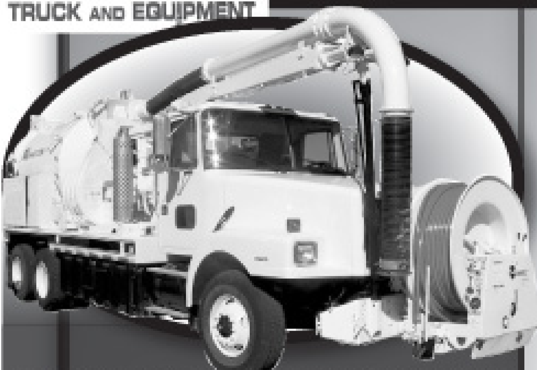
2001 Volvo Tandem Axel Vac-Con: V309SHA; Rear Engine: John Deere; 3 Stage Fan Unit; Bean pump: 80 GPM @ 2000 PSI; 600' 1" New Jetting Hose
