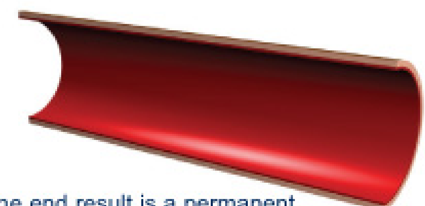
The end result is a permanent barrier between pipe and water
