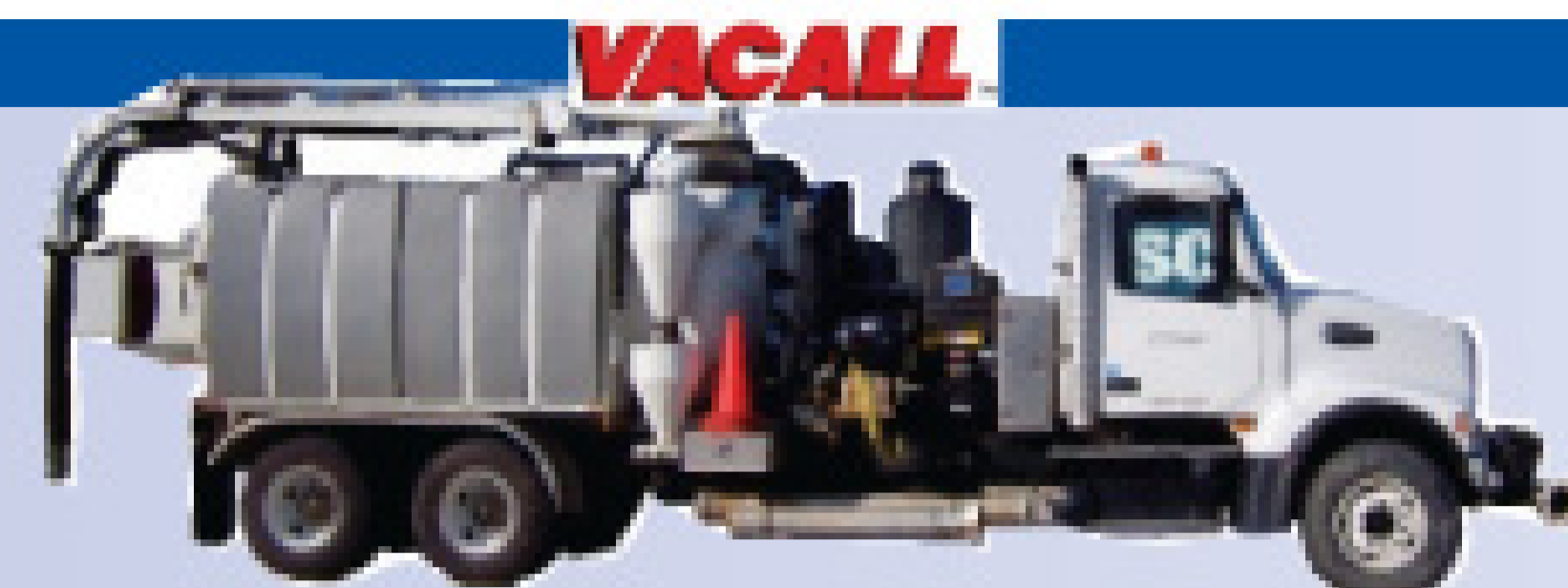
2006 Volvo VHD 64F, AquaTech B-12 Combination sewer Cleaner, Hydro-Excavation Package with Boiler, 20,000 Miles, 1700 Engine Hr., 220 Blower Hr., TS56 Hibon Blower, 310 Water pump hr., 65gpm @ 2500 psi
