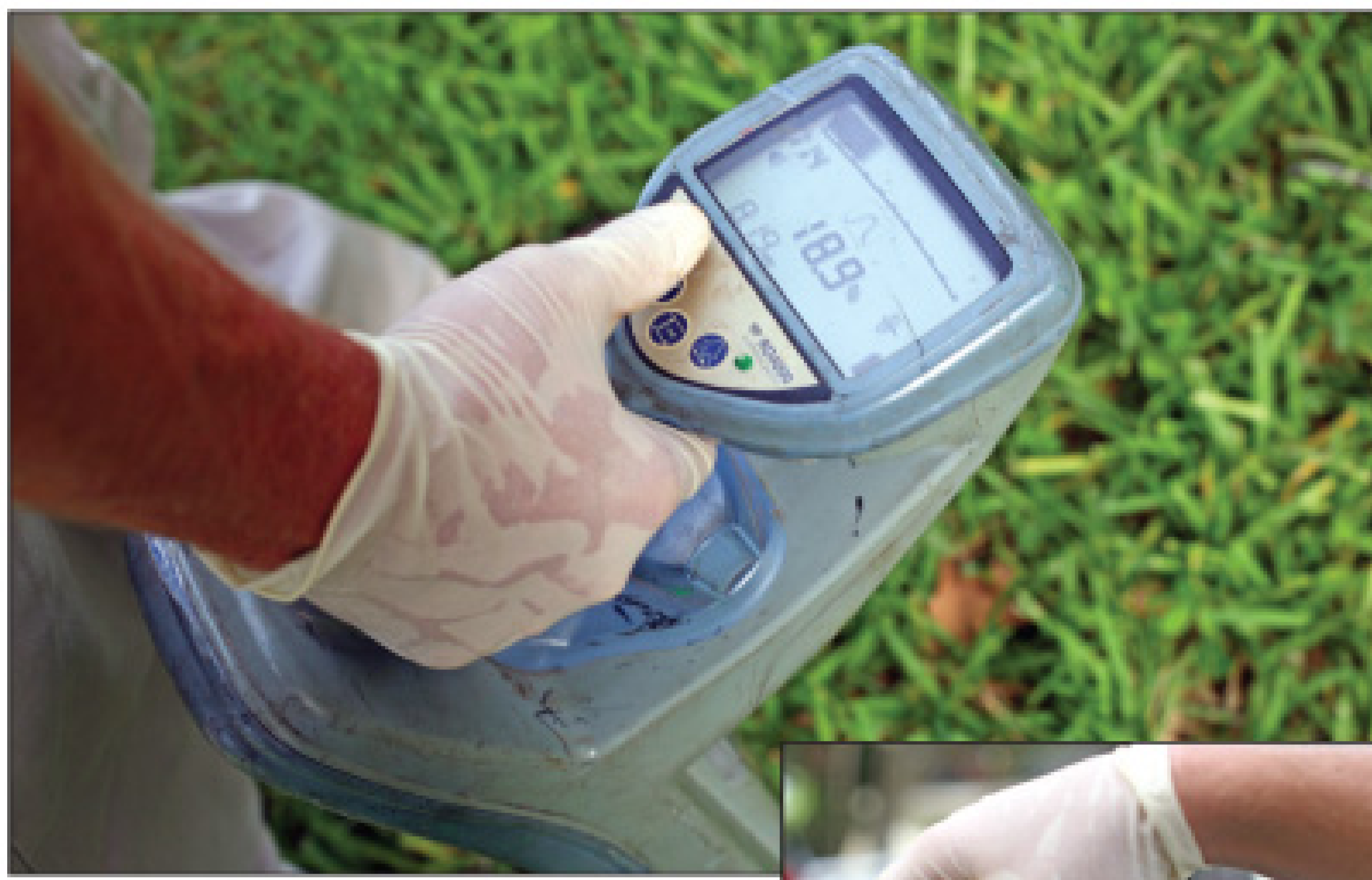
Above, Jerod Miller locates a camera in a pipe. At the right, Josh Miller uses a mobile digital video recorder to view images from a camera deployed in a lateral.
