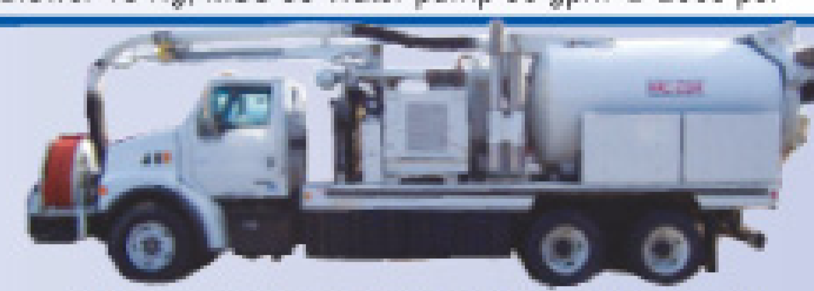
2004 Sterling LT7501, Vac-Con V312LHAE Combo. FMC-Bear Water pump 80 gpm @ 2000 psi, 16 cy, 13330 miles, 2230 Engine hr., 555 Auxilliary eng. Hr.
