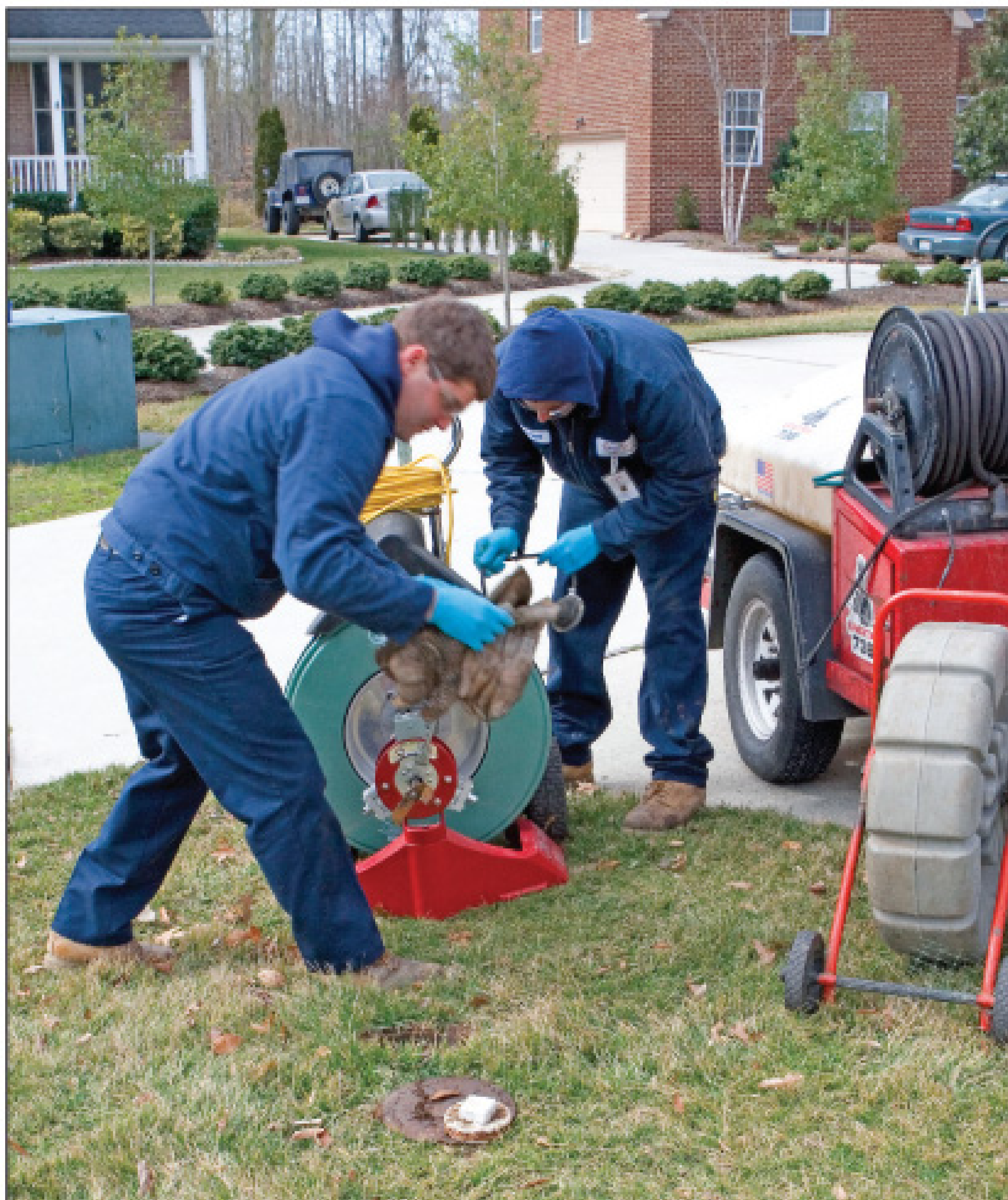
Paul Keane and Scott McCants prepare a Spartan 1065 mainline sewer machine for a lateral cleaning job.
