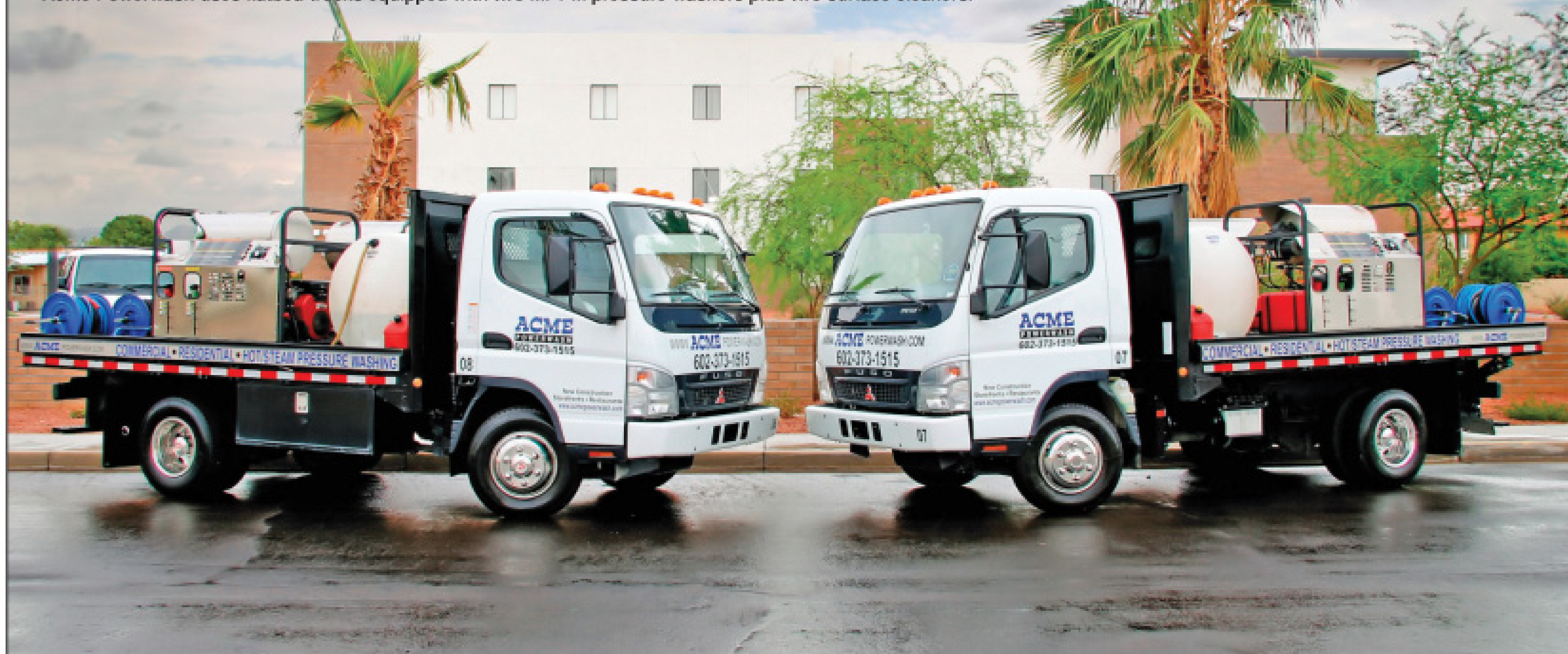
Acme Powerwash uses flatbed trucks equipped with two Mi-T-M pressure washers plus two surface cleaners.
