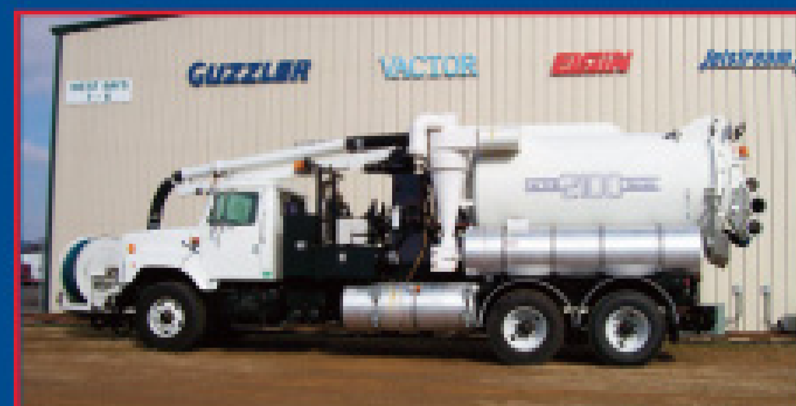
Unit #71134 2000 International Vactor 2110 Multi flow system, Roots 824 Blower READY TO WORK!
