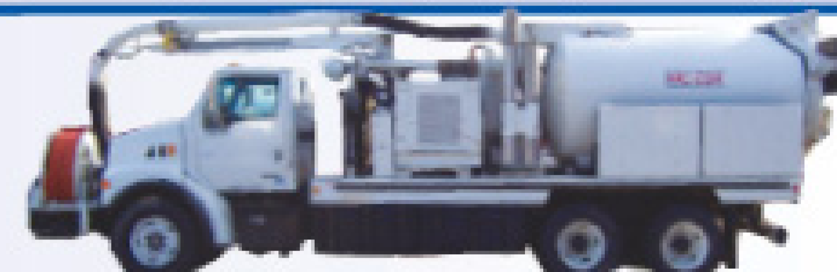
2004 Sterling LT7501, Vac-Con V312LHAE Combo. FMC-Bear Water pump 80 gpm @ 2000 psi, 16 cy, 13330 miles, 2230 Engine hr., 555 Auxilliary eng. Hr.
