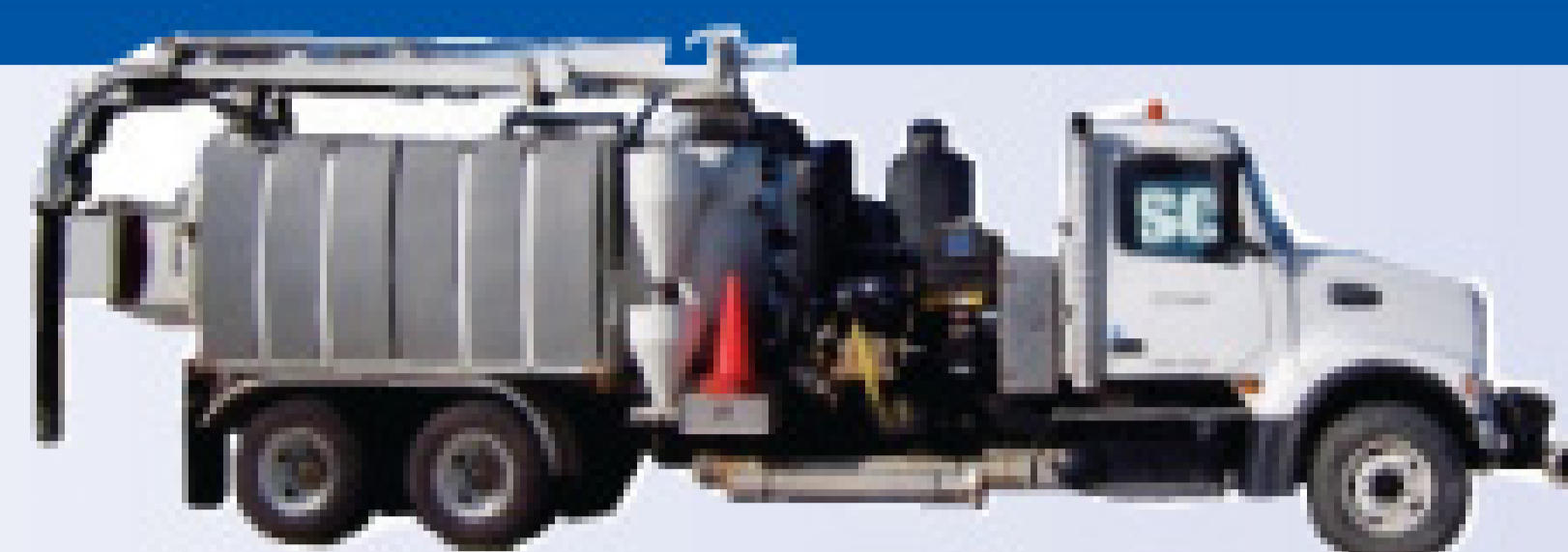
2006 Volvo VHD 64F, AquaTech B-12 Combination sewer Cleaner, Hydro-Excavation Package with Boiler, 20,000 Miles, 1700 Engine Hr., 220 Blower Hr., TS56 Hibon Blower, 310 Water pump hr., 65gpm @ 2500 psi
