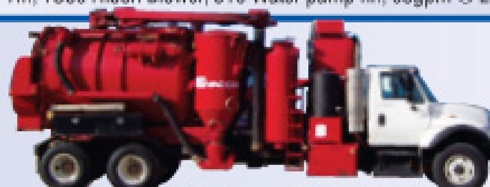
2005 International 7600, Vac-con 4716SMXD Hydro- Excavator, 16 cy Debris tank, 3000 psi @ 15 gpm cat 3560 73,370 miles, 2560 engine hr. 1175 blower hr. 1021 DVJ
