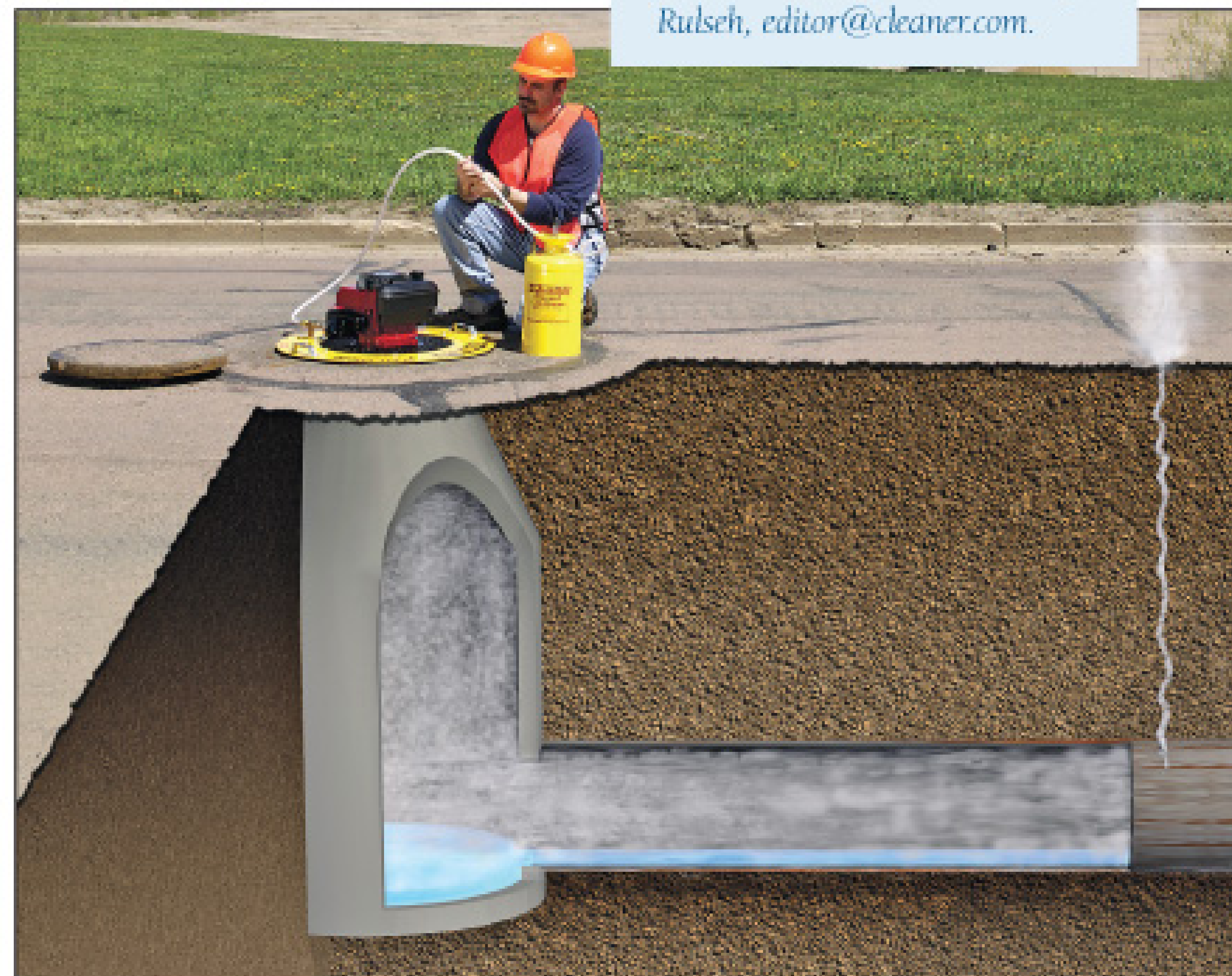
Smoke testing is a simple and reliable method of locating leaks in sewer systems. (Artwork courtesy of Hurco Technologies Inc.)
