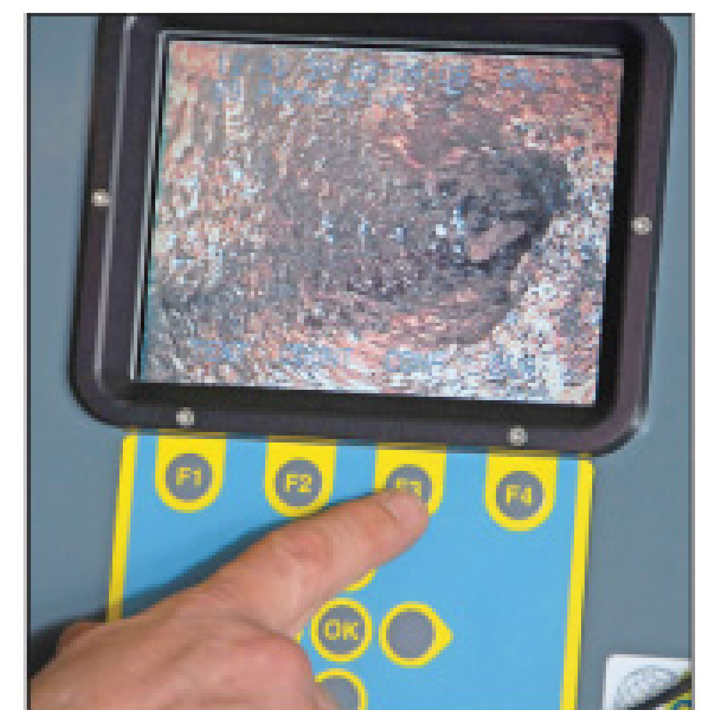
The Flexiprobe P330 monitor screen shows a pipe inspection in progress.
