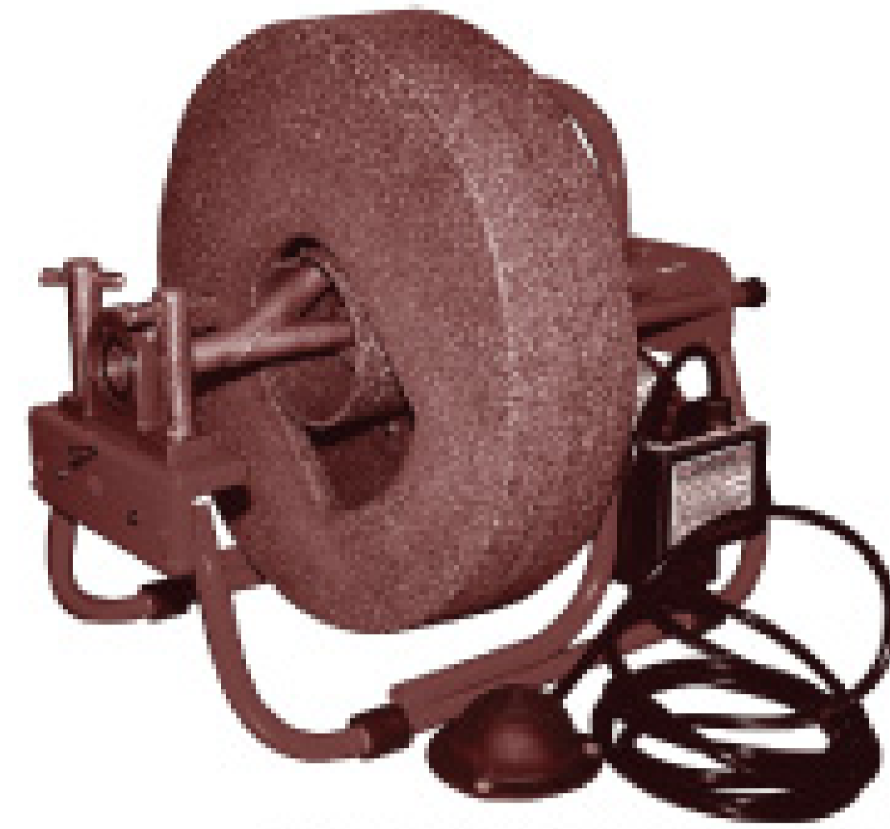
Above is - 1/4 HP motor, 230 rpm - The Esquire (DM138) machine!
