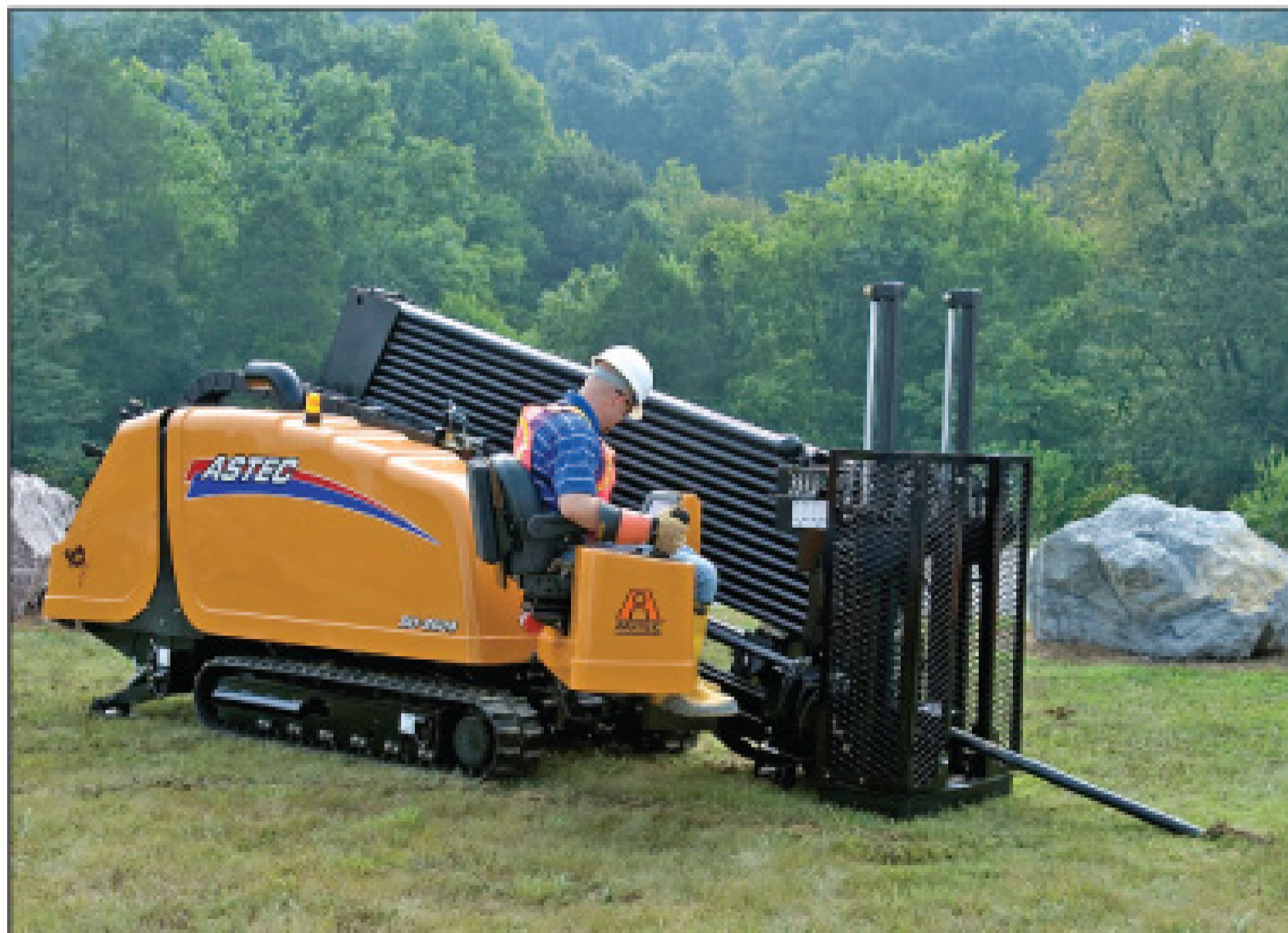
Astec EarthPro Series DD-2024 horizontal directional drill from Astec Underground
